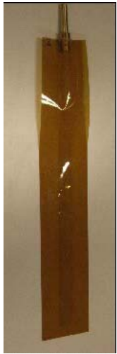
Kapton flexible radiators with "self rewetting" fluids
