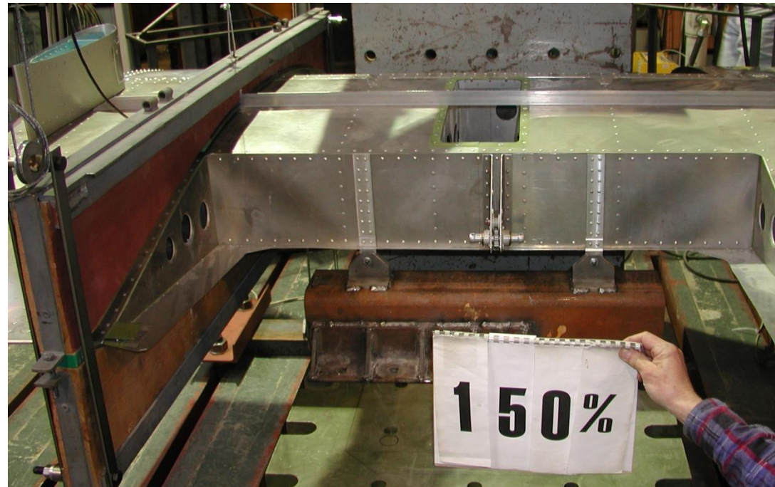
Centroplane torion test
