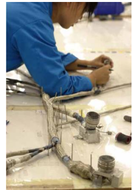
4. Printed drawing in wiring harness manufacturing
