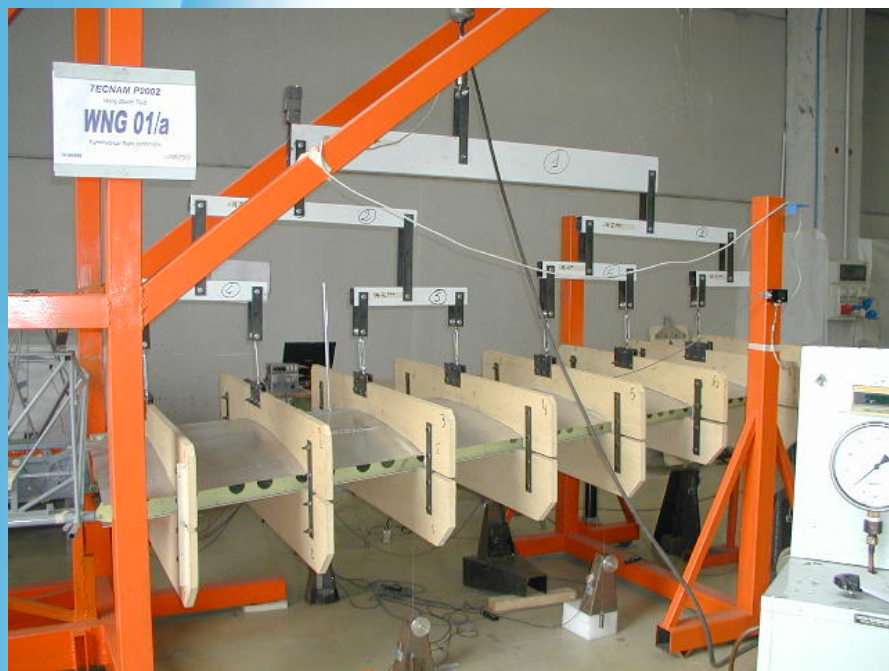
P2002JF Wing - Test Rig
