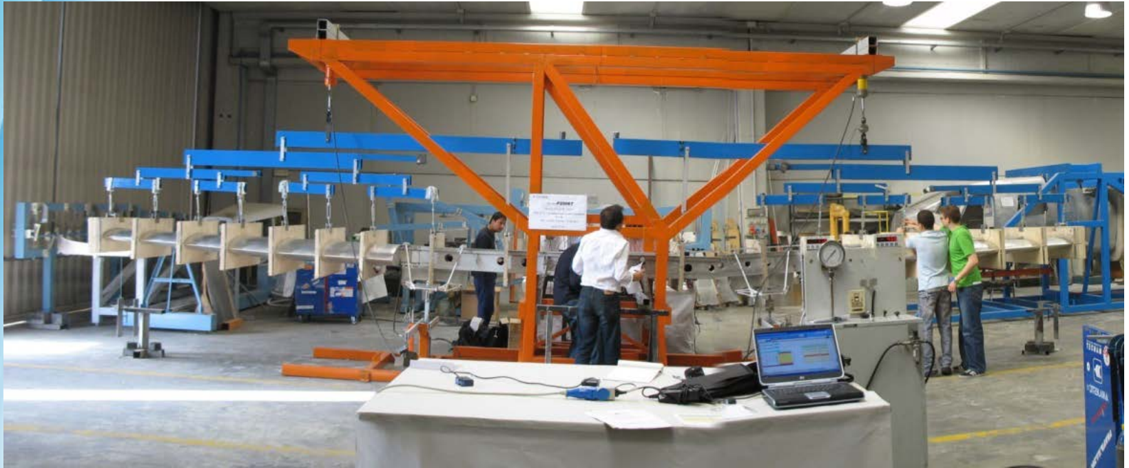
P2006T Wing Static Test - EASA CS 23 -
