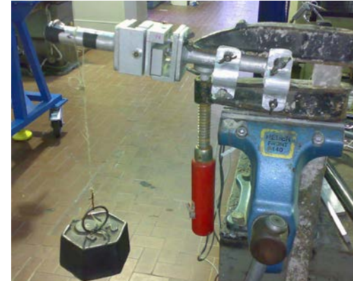
Load cell calibration. Then applied to the control stick
