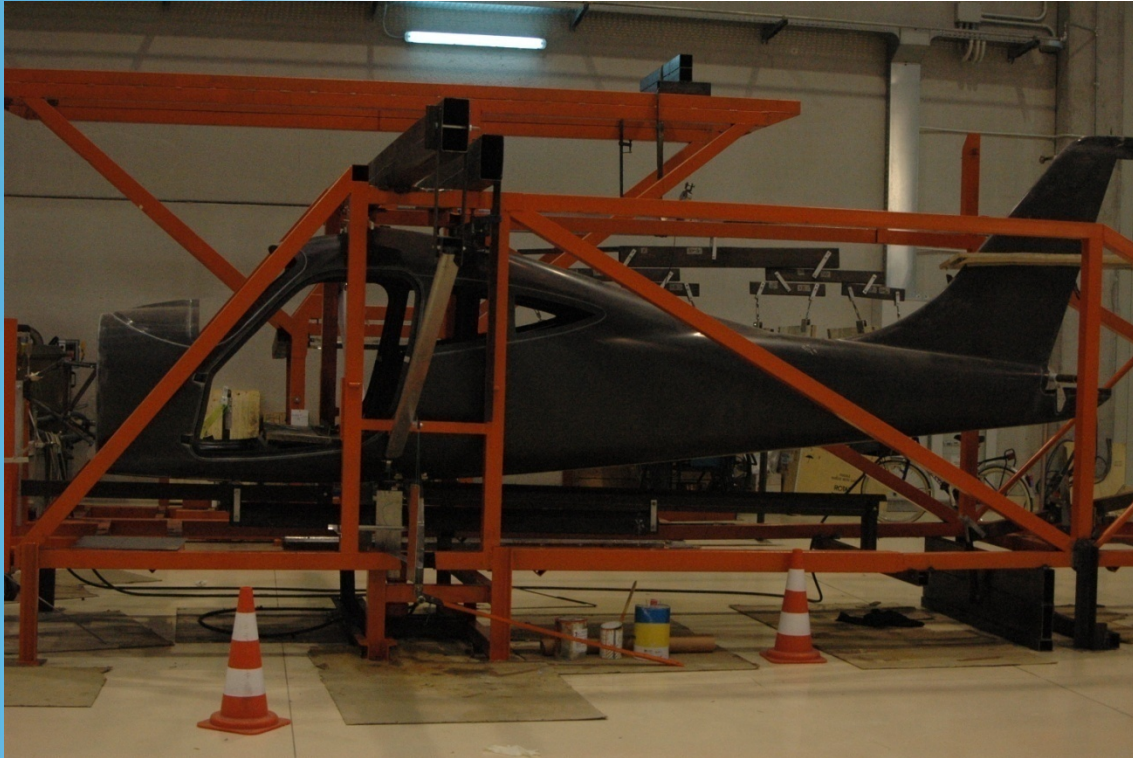
P2008 Composite Fuselage Static Test
