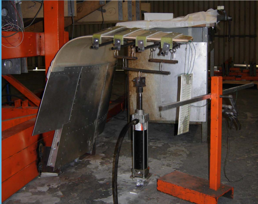
P2006T Composite Winglet Static Test - EASA CS 23 -
