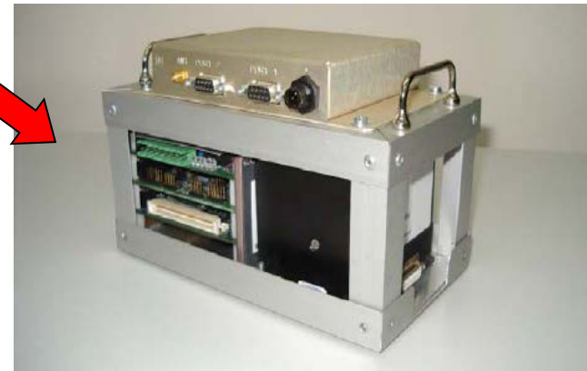
INS-GPS System (Micro Electro-Mechanical System for the inertial-satellite integrated navigation)
