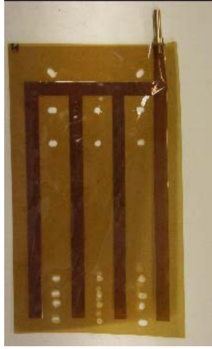
Kapton flexible radiators with "self rewetting" fluids
