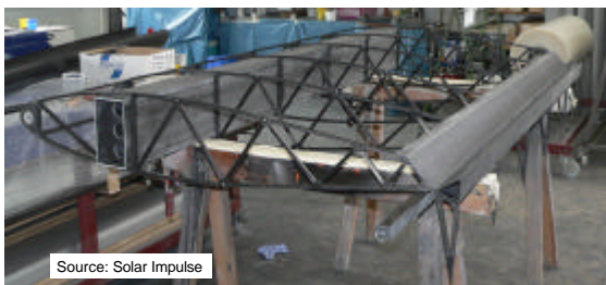
Fig. 5-16 Horizontal tail, rib spar arrangement
