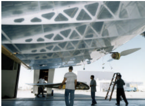
Abb. 4-13 Wing structure of the Pathfinder, AeroVironment
