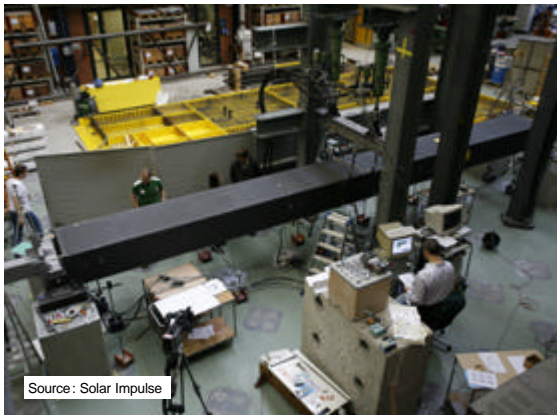
Fig. 5-15 Wing box, structural test
