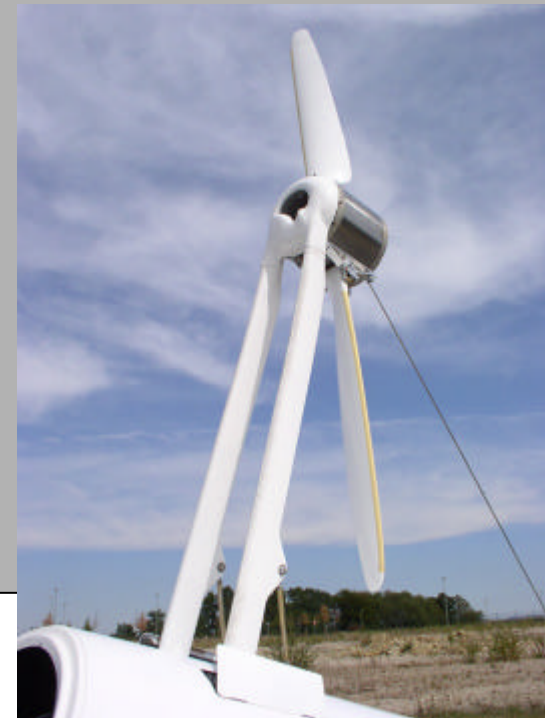
Motor for Antares Sailplane 42 KW, Propeller diameter 2m
