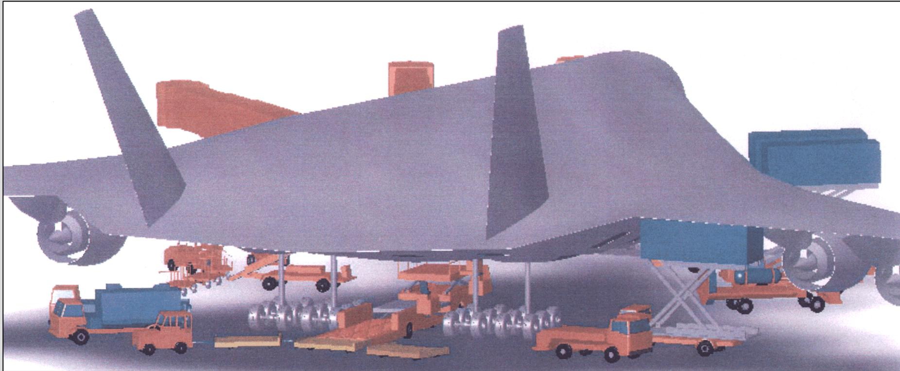
A **cargo loading** vehicle drives in between the MLGs. Cargo loading from below with lifting system.
