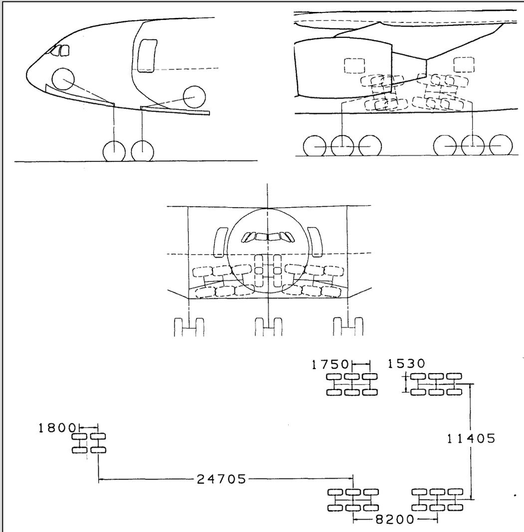
**Twin tandem (Bogie) nose landing gear.**
