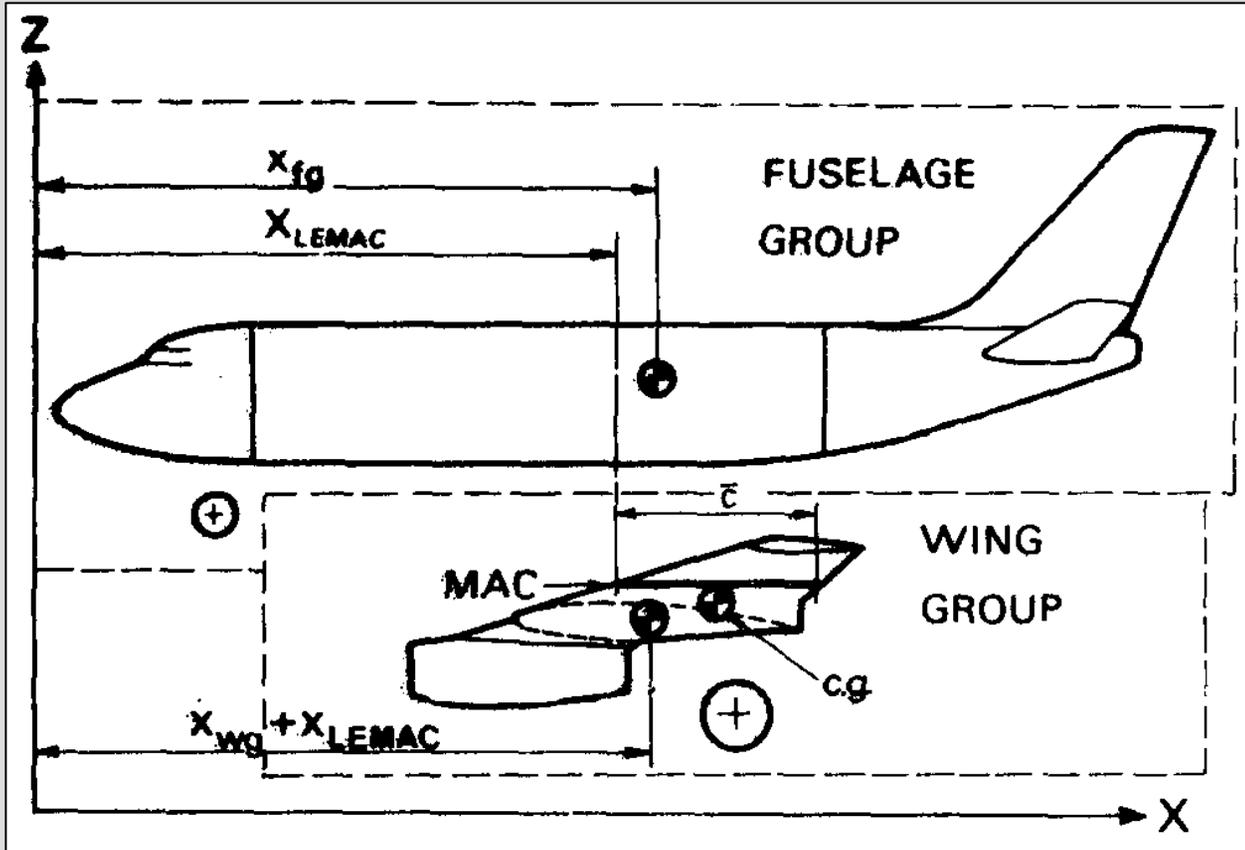
**Positioning of the CG on the Mean Aerodynamic Chord (MAC) for required static margin is achieved in conventional design by shifting the wing with respect to the fuselage. This approach is not possible in BWB design!**
