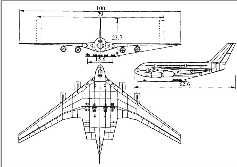
Best configuration from comparison of four New Large Aircraft configurations based on VELA specification.
