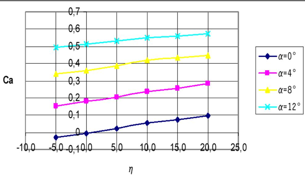
Lift coefficient dependend on flap angle
