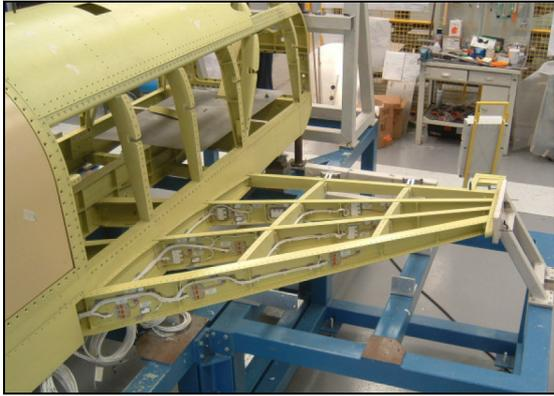
Figure 3. left semi-wing strain gauges
