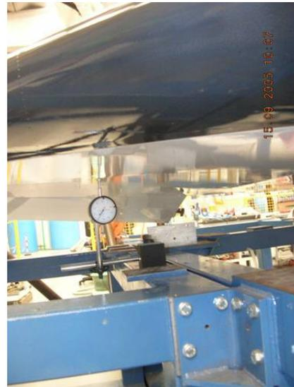
Figure 6. Analogical Dial Gauge mounted under left semi-wing.
