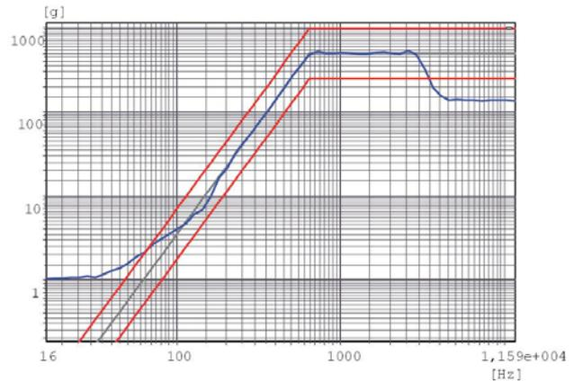
**Figure 13.** SRS produced by shaker.
