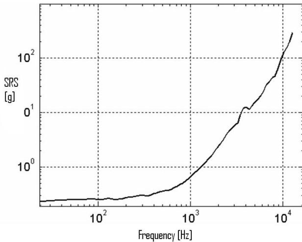
Figure 15. SRS produced with piezoceramics.
