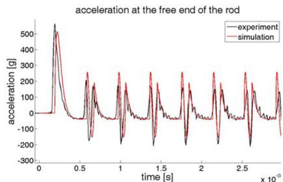
Figure 10. Acceleration at the free end of the rod.
