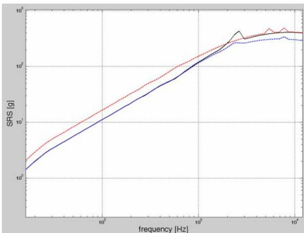
**Figure 12.** Variation of SRS: original SRS (black); sphere with increased mass (red); sphere with reduced elastic modulus (blue).
