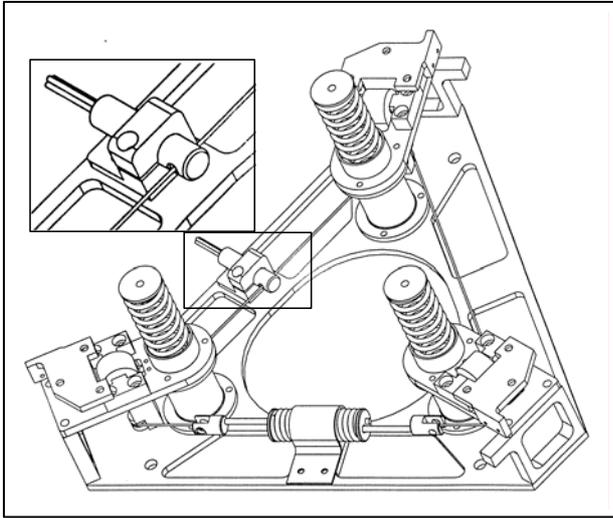
**Figure 3.** SSC micro satellite launch adapter with cable cutter.
