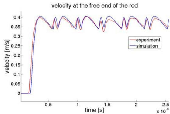
Figure 9. Velocity at the free end of the rod.
