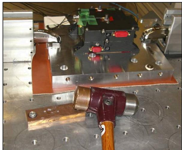
**Figure 6.** Freehand hammer on a MPS E-box [3].
