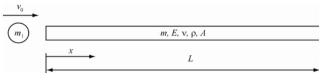
Figure 8. Impact of a sphere with rod.
