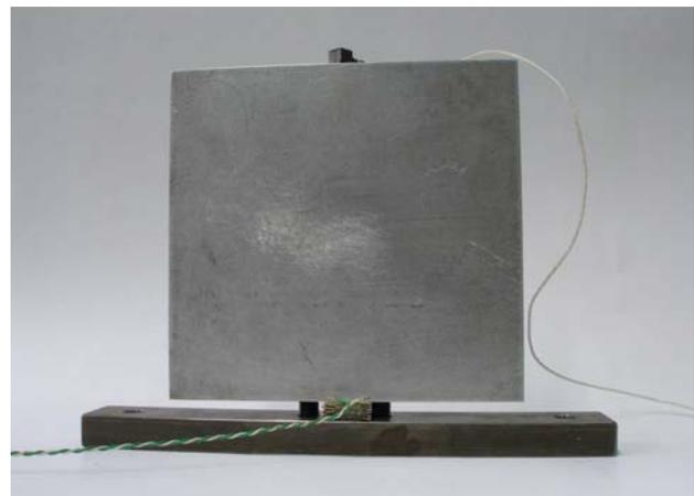
**Figure 14.** Piezoceramic actuator at bottom-side of a plate.
