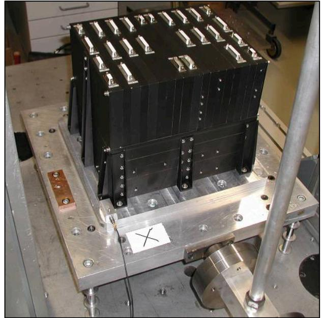
**Figure 5.** Pendulum hammer on an E-box (DLR).
