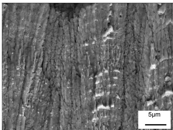
FIG 1. Cross-sectional microstructure of MSML
