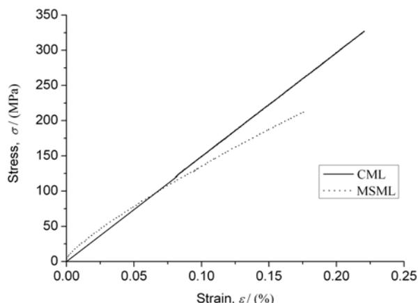
FIG 2. Stress-strain curves of NiCoCrAl / YSZ microlaminates
