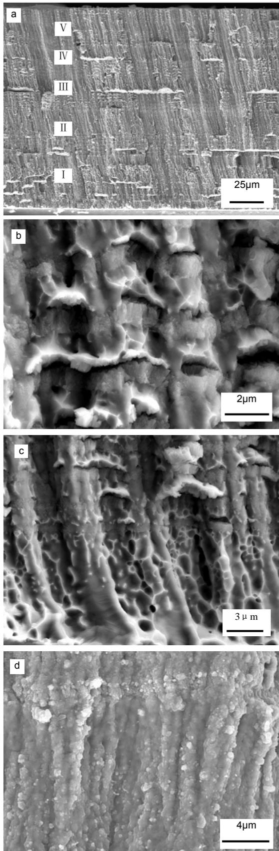
FIG 4. SEM micrographs of the fracture surfaces of MSML showing metal-layers with different
