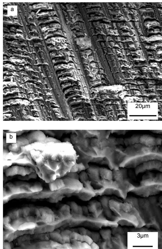
FIG 3. SEM micrographs of the fracture surfaces of CML tensile specimens tested at room temperature
