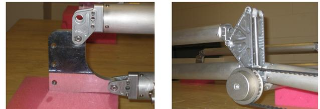
FIG 21. Prototype of the Six Bar Linkage
