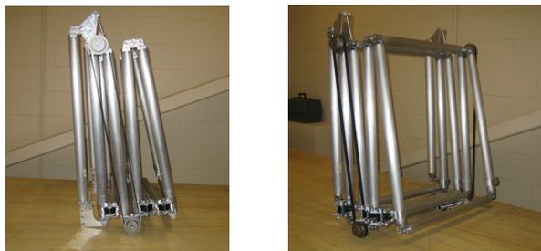
FIG 22. Antenna Frame Prototype (Stowed Configuration)
