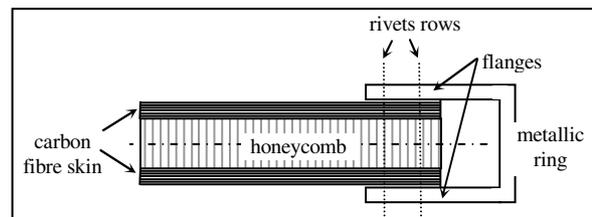
FIG 3. Lay-up sketch of a composite structure with a joint
