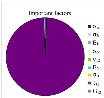
FIG 4. Important factors – 1<sup>st</sup> ply failure criterion
