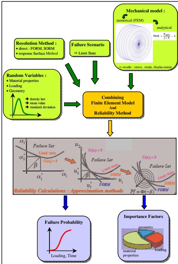
FIG 2. Combining Mechanical model and reliability method
