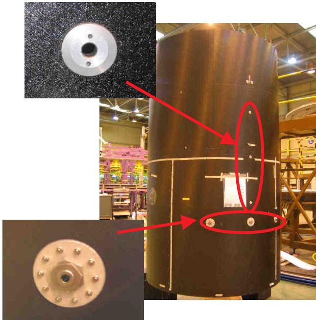
FIG. 14 Inserts installed in Central Tube.
