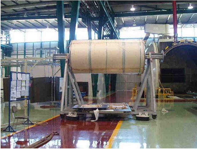
FIG. 8 Central tube on the mould after curing.
