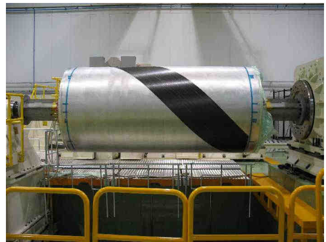
FIG. 6 Lay up of the first ply on the mould at the fibre Placement Machine.
