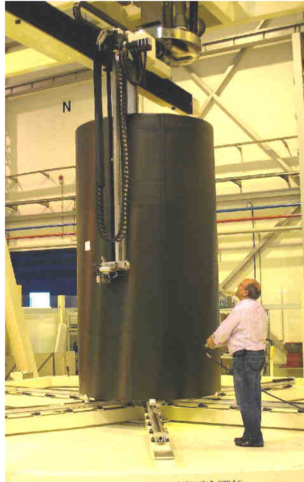
FIG. 15 Central Tube Shell automatic ultrasonic inspection.
