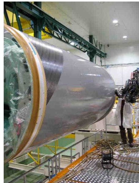
FIG. 7 Lay up of the first ply of the outer skin (over the core+adhesive) at the fibre Placement Machine.
