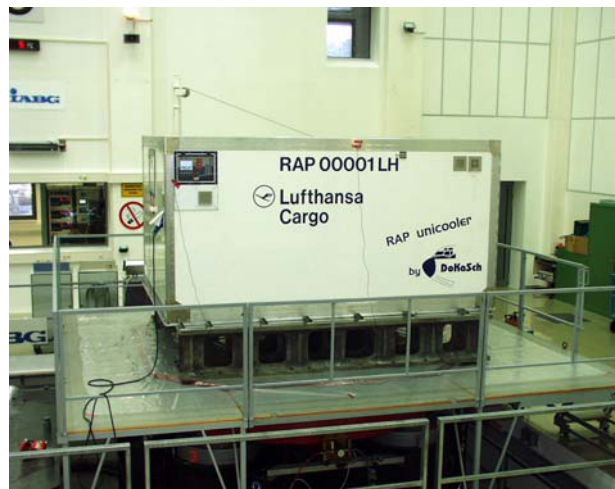
FIG 6. Vibration Test on a RAP Container Unicooler by DoKaSch on the 300kN Vibration System at IABG
