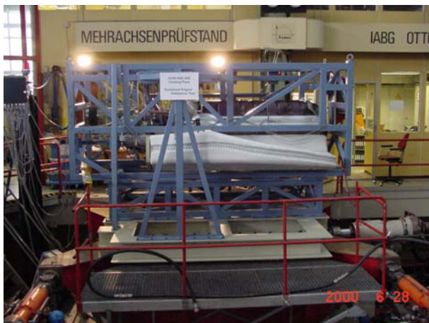
FIG 7. Vibration Test on a Main Landing Gear for a Commuter Aircraft by Liebherr on the 300kN Vibration System at IABG
