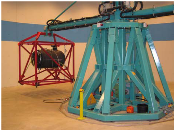
FIG 3. Acceleration Test on a Waste Water Tank by AOA on the Centrifuge at ZARM
