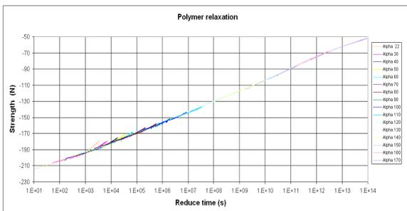
**FIG. 11: Residual strength versus reduced time**
