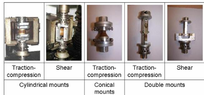
**FIG. 3: Tested mounts**
