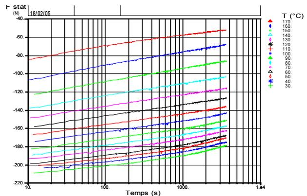
FIG. 9: Measurement of static strength at different temperatures
