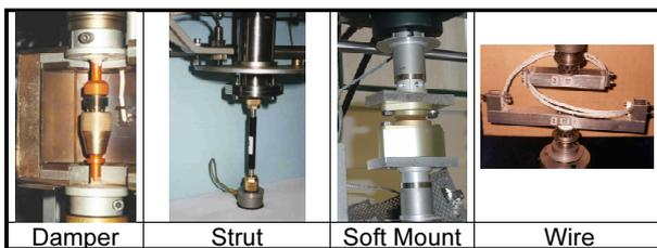
**FIG. 2: Measurement of devices with VISCOANALYZER**
