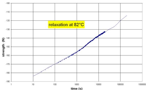
**FIG. 12: Experimental residual strength after 4 days**
