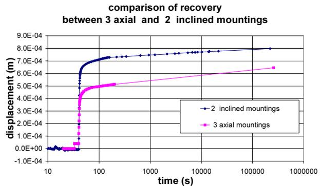
FIG. 7: Displacement recovery
