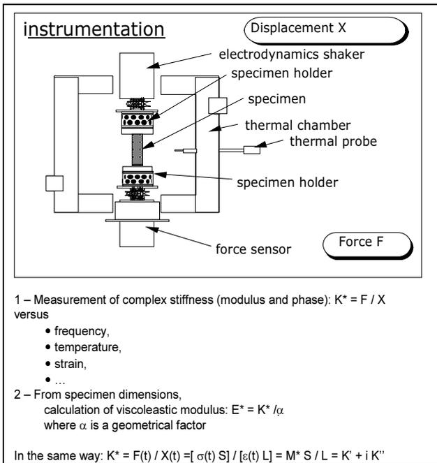
**FIG. 1: Principle of measurement of VISCOANALYZER**
