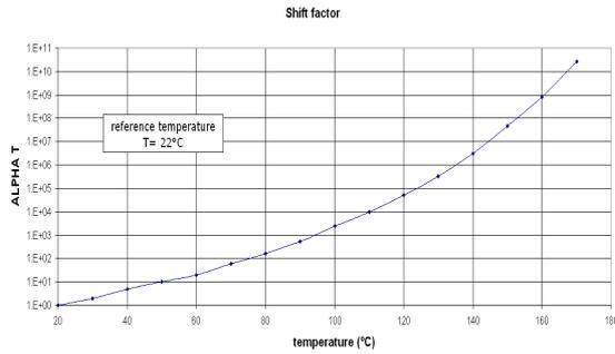
**FIG. 10: Calculation of shift factor at different temperatures**
