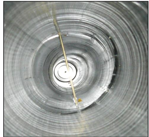
**FIG. 13 View inside boom with DEA-SCE embedded**
