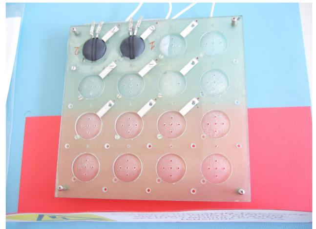
**FIG. 14 Bubble matrix breadboard, partly equipped with actuators**
