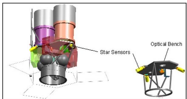
FIG 9: Star Sensors implemented on Optical Bench
