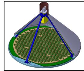
FIG 11: Antenna with Pointing Mechanism
