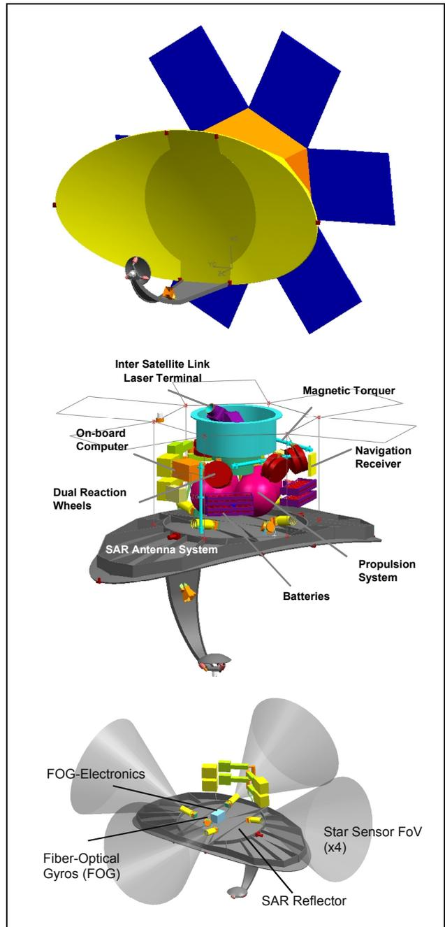
FIG 6: OHB-System Satellite Solution for a Future High Resolution SAR Mission
