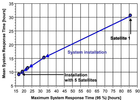
FIG 5: Improvement of the System Response Time by the Implementation of Multiple Satellites
