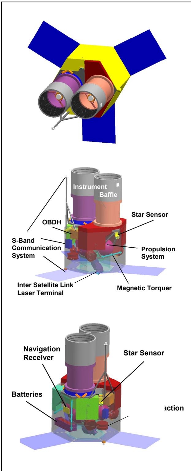
FIG 7: OHB-System Satellite Solution for a Future High Resolution Optical Mission
