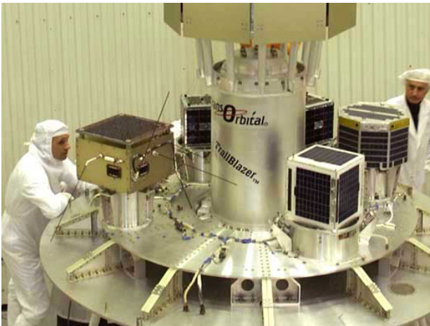
FIG 1 Rubin 2 (left) integrated on the Dnepr adapter ring
