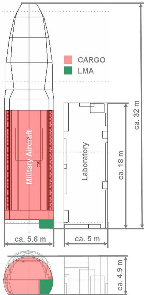
FIG 5. Comparison of dimensions of aircraft cavity and laboratory at HSU-HH
