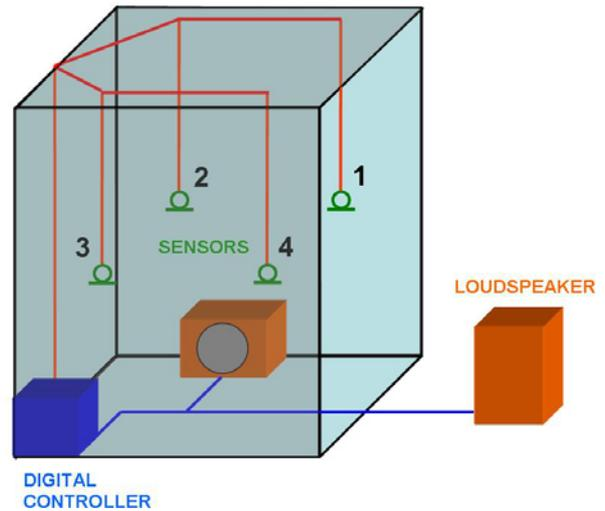
FIG 8. Outline of test bed for primary field synthesis
