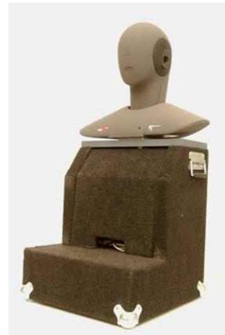
FIG 6. Dummy of loadmaster torso and head
