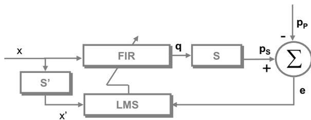
FIG 7. FxLMS algorithm for primary field synthesis
