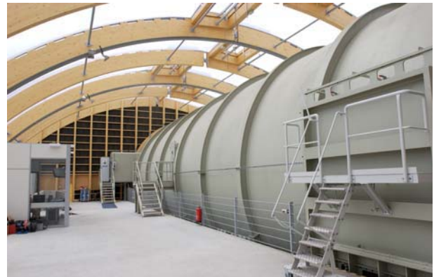
Figure 2: Low-pressure chamber of the Flight Test Facility. © Fraunhofer/Bernd Müller
