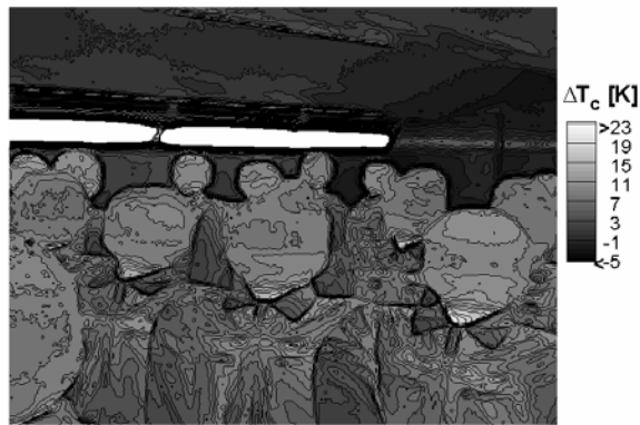
FIG. 2. Snapshot of the surface temperature differences with respect to the mean cabin temperature of passenger dummies and the cabin measured by infrared thermography for configuration A 50/50.
