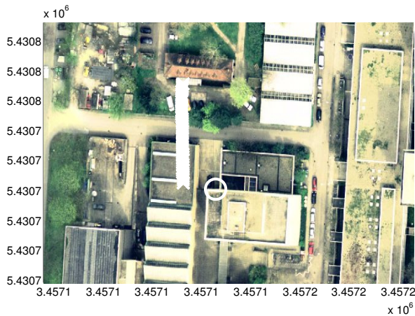
Fig. 12. Geo-located corner of house from Fig. 11; the estimated position is marked with a white circle, the positions of the MAV are marked with white crosses.
