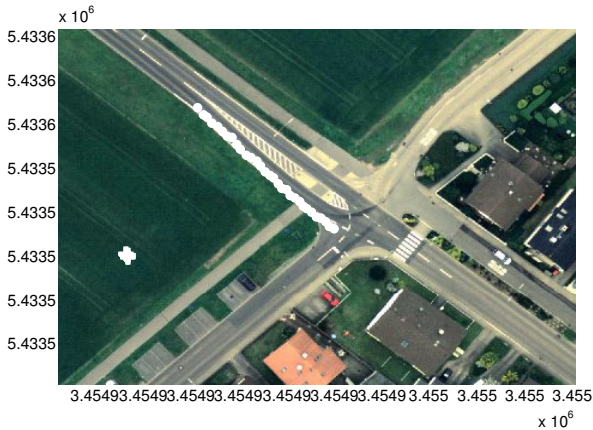
Fig. 10. Geo-located trajectory of the tracked object in Fig. 9, the mean position of the used MAV is marked with a white cross.
