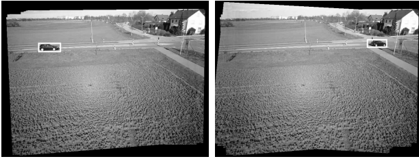
Fig. 9. Two frames of a stabilized image sequence with the detected and tracked object that is marked with white boxes.
