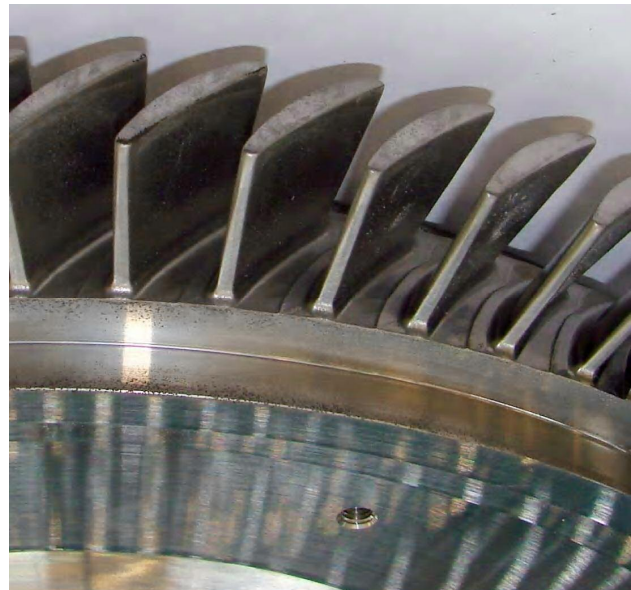
Fig. 12: Airfoils rough-machined using ECM
