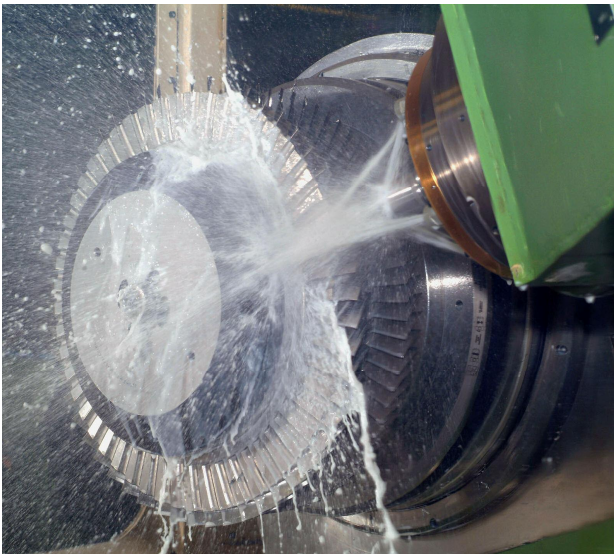
▲ Fig. 8: Blisk machining on a five-axis milling machine
