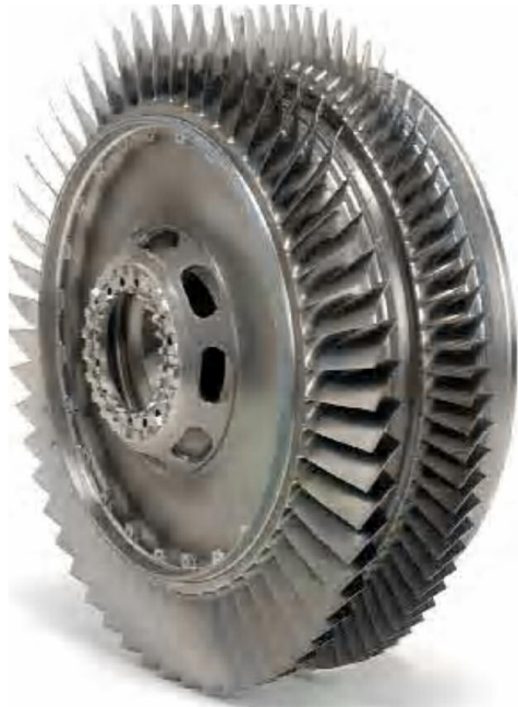
▲ Fig 19: High-pressure compressor blisk drum
