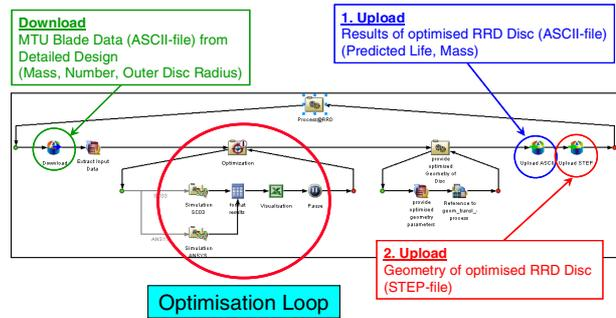
FIG 7. Local optimisation process at Disc 2 design partner. up- and download of data is automated.
