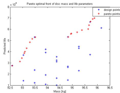
FIG 14. Pareto front (red points) of lifing and weight objectives. Note that disc designs with mass between 93.5 and 95 kg do not comply with the minimum lifing constraint of 40000 flight cycles causing a discontinuous Pareto front. The blue points depict the design space sampling.
