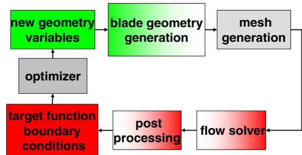
FIG 2. Process chart of the 3D blade shape optimisation.
