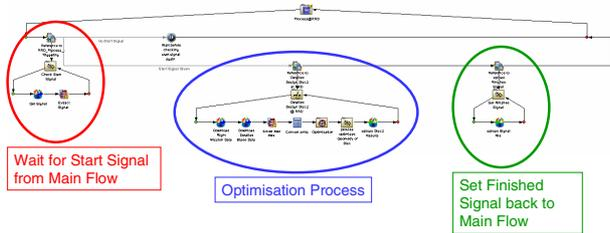
FIG 6. Partner's design framework for multi disciplinary optimisation and robust design of Disc 2. Trigger-components are used for starting and finishing the local design process
