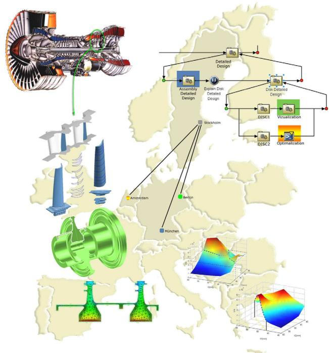
FIG 1. Multi-partner multi-site virtual enterprise collaboration for an engine multidisciplinary design analysis process.
