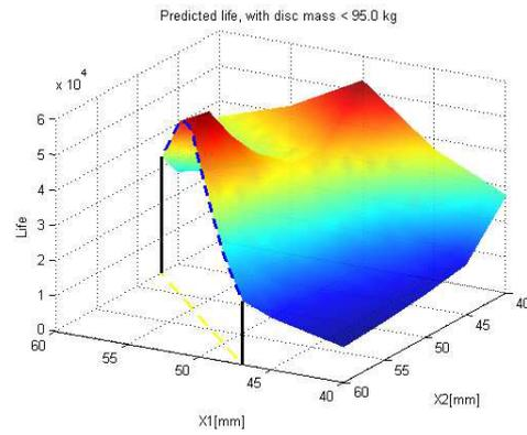
FIG 13. Calculated lifing in engine disc design space. The feasible design space satisfies the maximum disc weight constraint.
