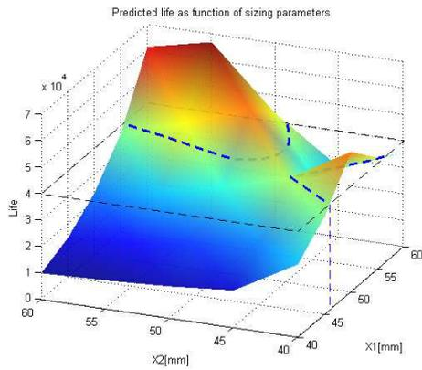
FIG 12. Calculated lifing in engine disc design space. The part above the waterline satisfies the minimum lifing constraint (40000 flight cycles).
