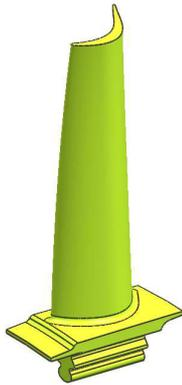
FIG 3. Optimised blade completed with platform and fir tree.
