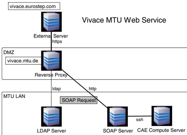
FIG 4. Prototype Security Infrastructure
