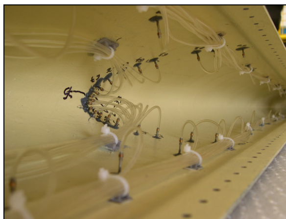
FIG. 10. Internal view of the wing leading edge with the pressure taps metallic inserts and pneumatic tubing
