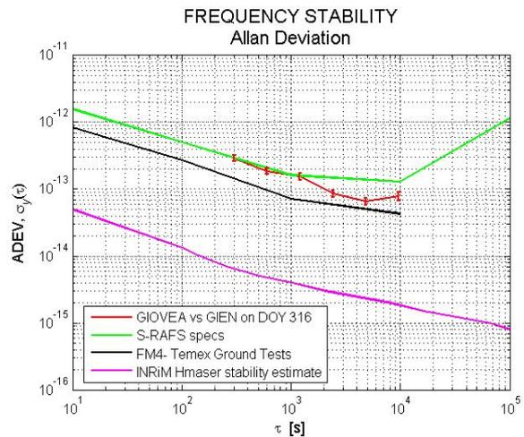
FIG 11. Stability of the GIOVE-A "apparent" clock with respect to the GIEN master clock on a "quite" day (no anomalous behaviour)
