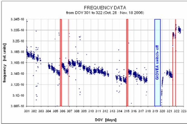
FIG 12. GIOVE-A “apparent” clock frequency from 28.10.06 – 18.11.06. Frequency jumps are indicated by red lines.
