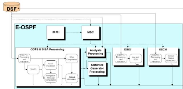
FIG 8. E-OSPF functional diagram
