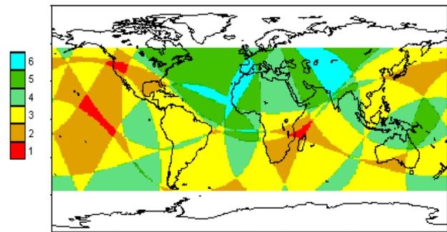
FIG 3. Depth-Of-Coverage (DOC) for the 13-station network.
