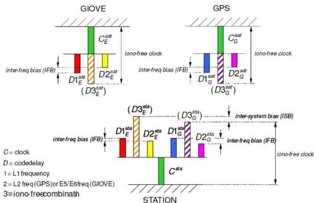
FIG 9. Relationships between GIOVE and GPS station signal-path delays.
