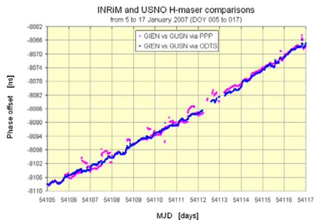
FIG 17. Phase offsets between the active hydrogen maser clocks at INRiM (GIEN) and USNO (GUSN), January 5-17, 2007, computed using precise point positioning (PPP) and the ODTs software.
