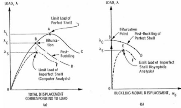
FIG 3. Load-deflection curves showing limit and bifurcation points. a) general nonlinear analysis, b) asymptotic analysis
