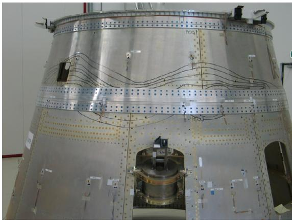
FIG 8. Deformed Interstage 1/2 structure after failure due to general buckling. (Each contour line represents 0.5mm deformation)
