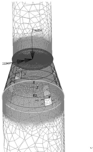
FIG 6. FE model of IS1/2 and adjacent structures showing load application of axial thrust load and bending moment.
