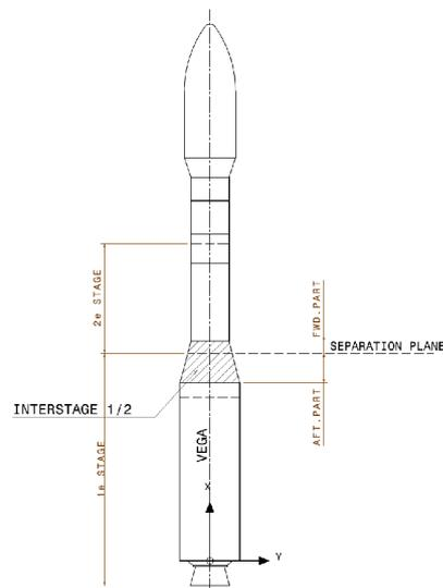
FIG 1. Vega Launch Vehicle showing position of Interstage 1/2
