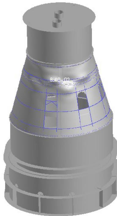
FIG 9. Analysis result for general buckling of IS 1/2 in test configuration (correlated FE model)
