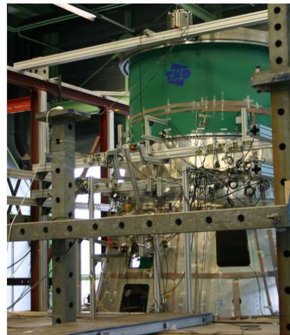
FIG 7. Interstage 1/2 qualification model in test set-up
