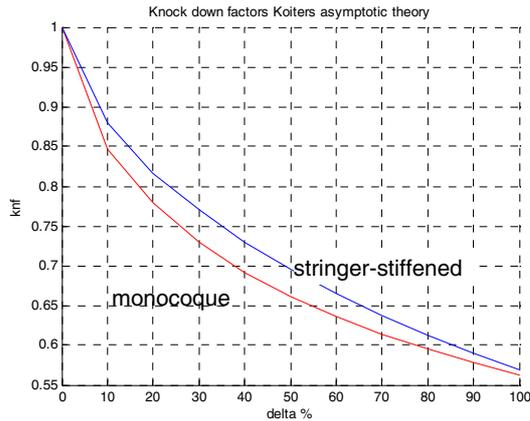
FIG 5. Comparison imperfection sensitivity monocoque and stringer stiffened shell
