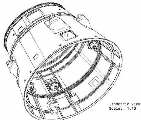
FIG 2. Geometrical model of Interstage 1/2
