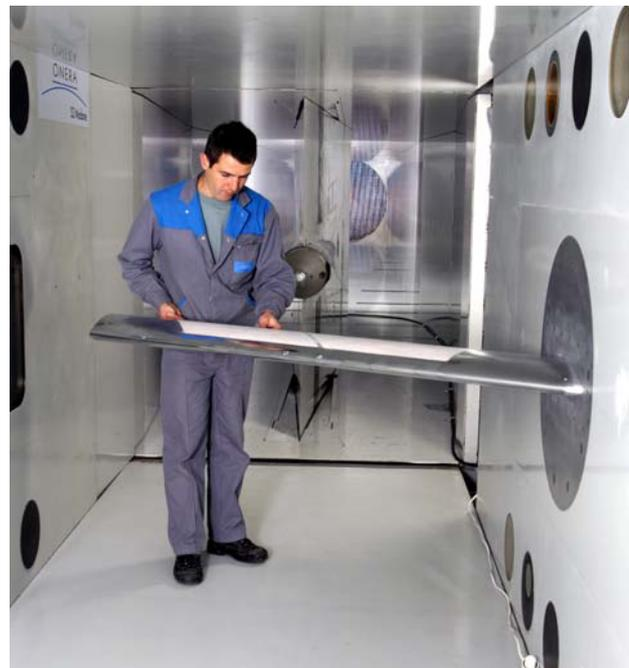
FIG. 4- Swept wing model in the S2MA wind tunnel.
