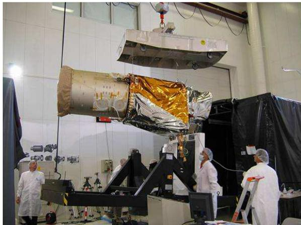
dit CNES: Fig. 1: integration of the COROT telescope at CNES
