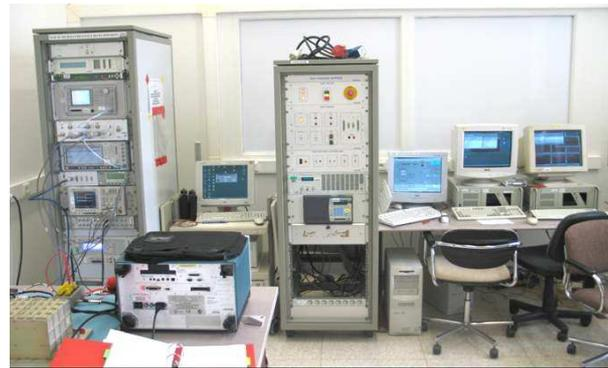
Fig. 5: the EGSE for MYRIADE Micro satellites
