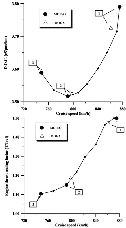
FIG. 10 Examples of cruise speed effect on aircraft characteristics (OEW, DOC, block fuel and engine thrust scaling factor). Comparison between max cruise speed (1), min D.O.C. (2) and min cruise speed (3) optimized configurations obtained by MOPSO procedure and a genetic-based multi-objective optimizer (MOGA)
