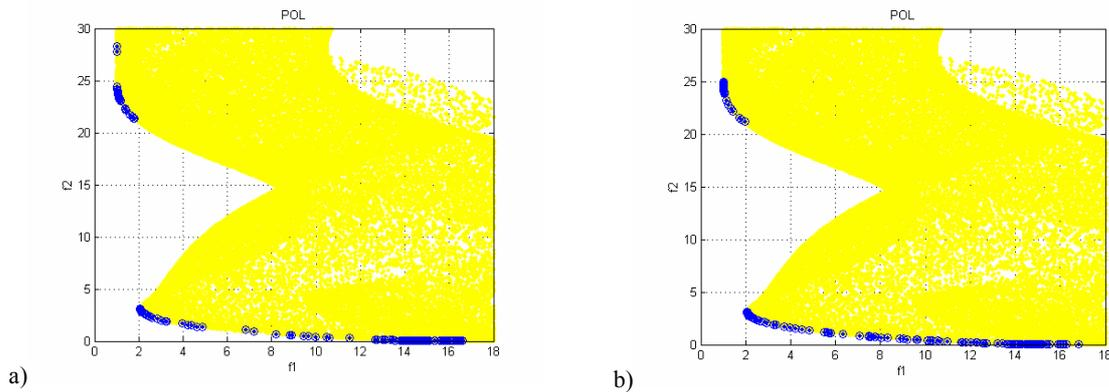
FIG. 4 MOPSO application to POL problem: a) without sampling density implementation; b) with sampling density implementation
