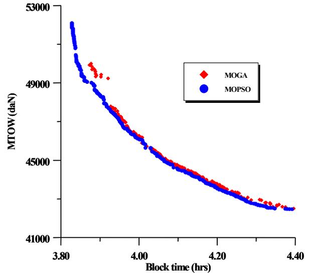
FIG. 7 Comparison between Pareto curves obtained by MOPSO procedure and a genetic-based multi-objective optimizer (MOGA)
