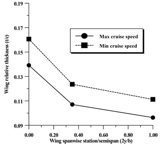
FIG. 9 Wing relative thickness related to max cruise and min cruise speed optimum configuration
