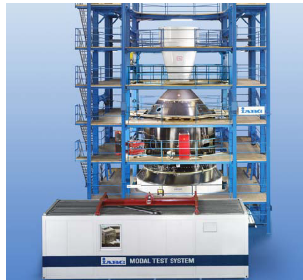
Fig. 2: Already History: IABG's Modal Test Container as used for many ARIANE 5 modal tests
