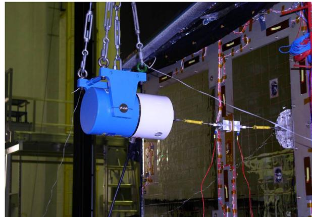
FIG 13 Minishaker for microvibration test
