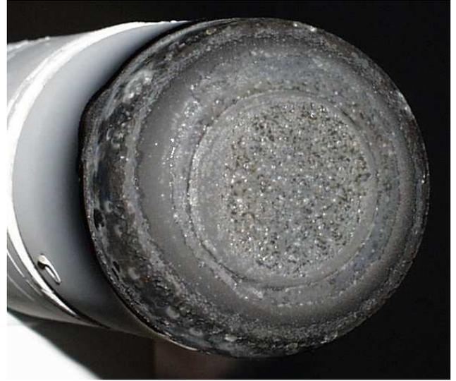
Figure 5 SSIC-sample and cap after test in oxygen plasma flow at  $p_{ch}=3000$  Pa
