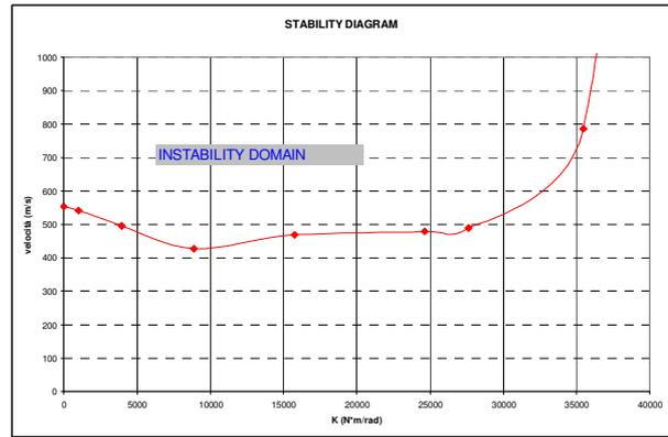
Fig. 8: Flight speed vs elevon control circuit stiffness
