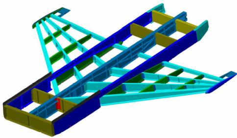
Fig. 3: USV wing structure
