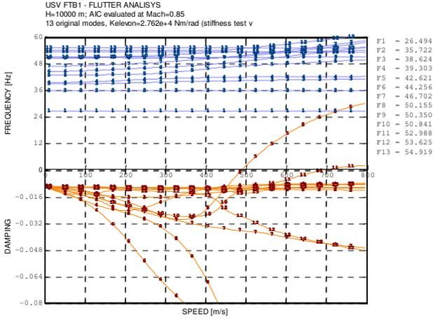
Fig. 5: v-g diagram for USV
