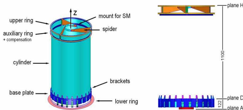
Figure 6. Structure of a Cassegrain telescope and definition of planes on the position of the primary mirror (D), secondary mirror (H) and camera (A).
