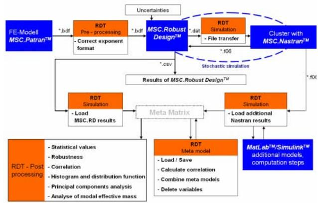
Figure 4. Flowchart of the Robust Design Toolbox (RDT) with its four parts: pre-processing, simulation, meta model and post processing.
