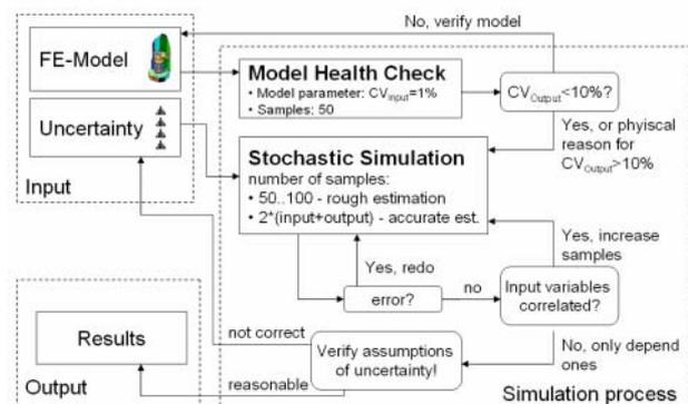
Figure 1. Main steps of a full stochastic simulation process.
