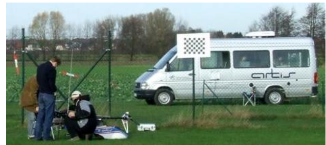
FIG. 14: Preparing a helicopter flight. In the background, there is a chessboard pattern for camera calibration and the ground control station truck.
