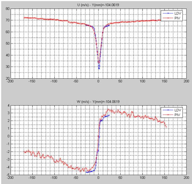
Fig. 10 : Mean velocity profiles (PIV at CEPRA19 and LDV in F2)
