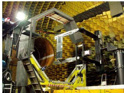
Fig. 6: Second PIV rig - Double octagon
