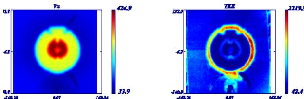
Fig. 12 : Mean axial velocity and turbulent kinetic energy for  $X/D = 1$
