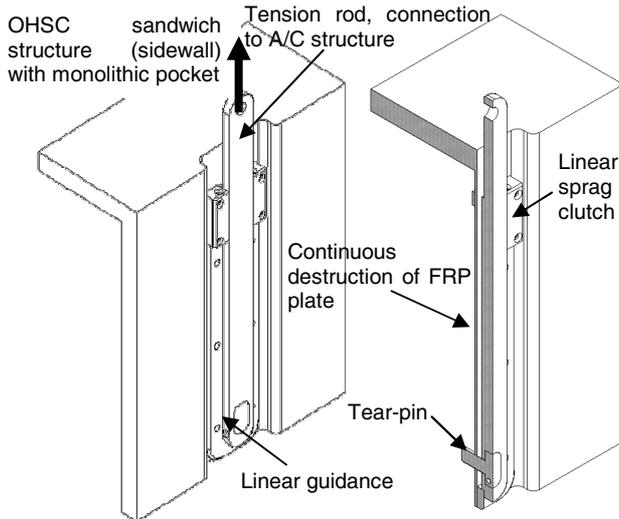
FIG 2. Pin/plate-absorber concept with part of an OHSC sandwich structure (patent pending)
