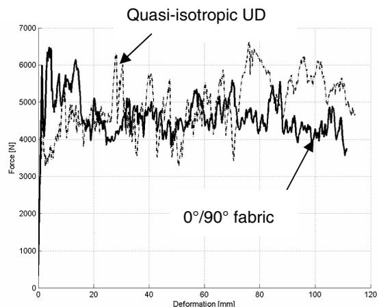
FIG 4. Force-deflection curves of  $0^{\circ}/90^{\circ}$  fabric (solid) and quasi-isotropic UD specimens (dash-dot)
