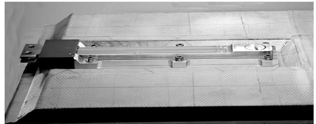
FIG 7. Integrated pin/plate absorber in a sandwich panel
