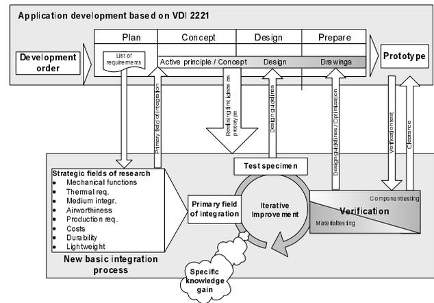
FIG 9. Development process to integration of functions.
