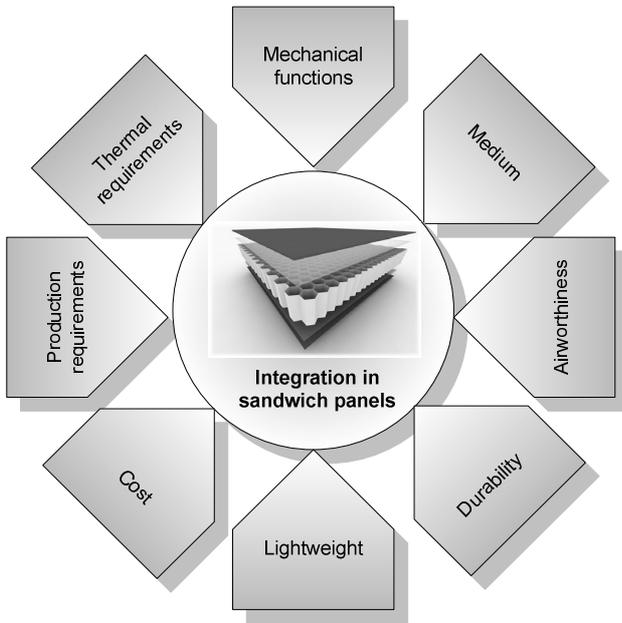
FIG 8. Influences on the integration of medium and functions in sandwich panels.
