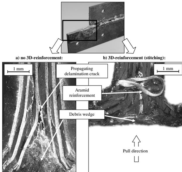
FIG 5. Micrographs of CF/EP specimens: a) 0°/90° fabric, b) 0°/90° fabric 3D-reinforced
