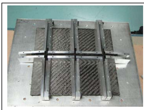
FIG. 5.3.h: Tooling of Cross ribs feet/skin attachment panel just before pinning operation
