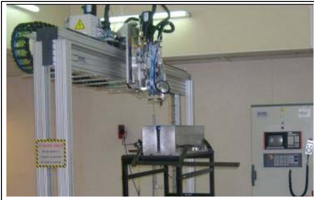
FIG. 5.1.a: EADS Innovation works Z-pinning machine
