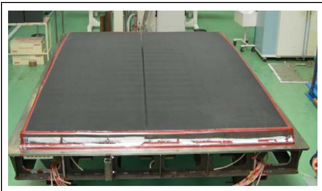
FIG. 3.3.a: FP6 ALCAS program Central Wing Box extrados panel made of LRI VAP technology (AIRBUS France in cooperation with EADS Innovation Works)
