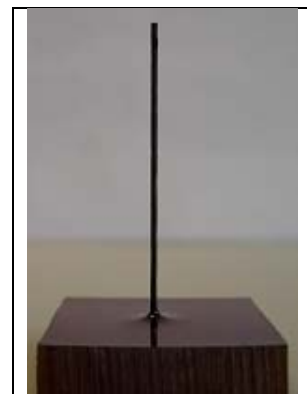
FIG. 5.2.c: Pull out test pin specimen for a pin of 0.7mm (LMS ISAE). On this picture, the pin is implanted in a resin plate.
