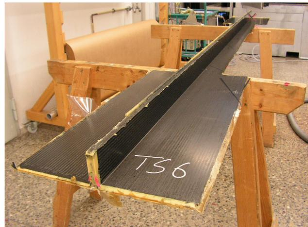
Fig. 15: Successfully Infused Raw Stringer (Laminate A)
