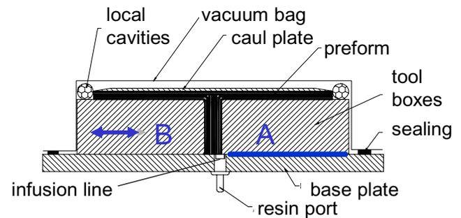
Fig. 11: Mould Design for Full Scale Prototypes
