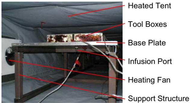
Fig. 13: Mould in Heated Tent
