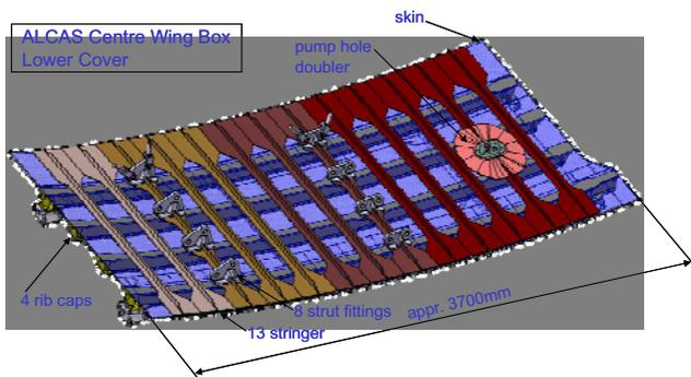
Fig. 4: ALCAS CWB Lower Cover Components
