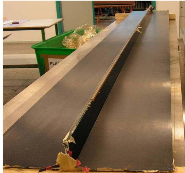
Fig. 14: Successfully Infused Raw Stringer (Laminate B)
