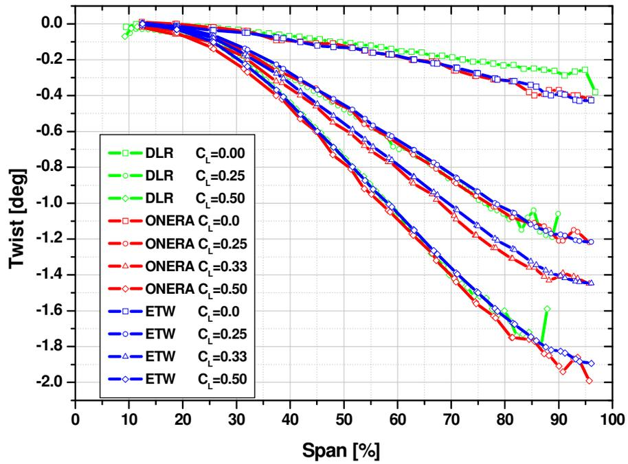
Fig.1 MDM Measurements obtained during the EWA Workshop at ETW.
