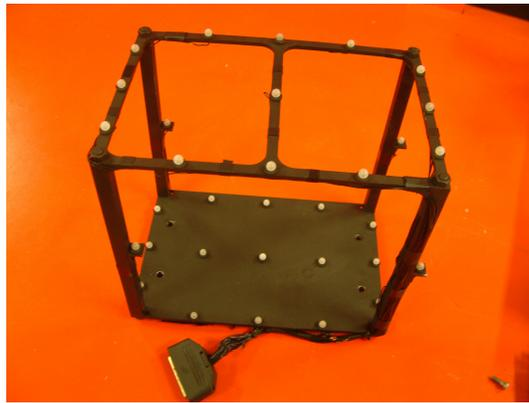
**Fig. 11. ETW Calibration Frame**
