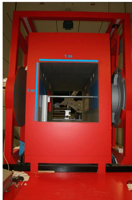
**Fig. 7. Dummy TWG Working Section at DLR, Göttingen.**
