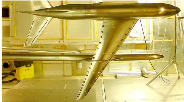
**Fig. 4. ETW System showing the attached markers on the main wing and HTP.**
