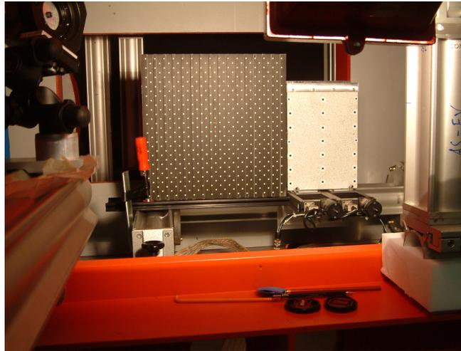
**Fig. 10. DLR Calibration Plate Mounted Next to Test Plate**
