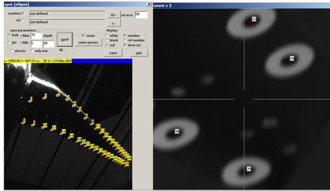
**Fig. 5. Marker detection using the ONERA System**
