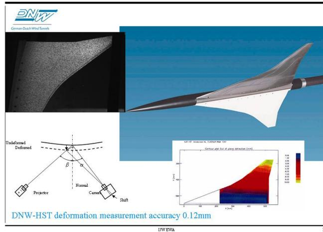
**Fig. 3. DNW Projected Pattern Method**
