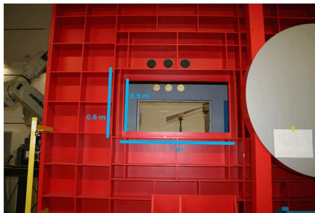
**Fig. 6. Dummy TWG Working Section at DLR, Göttingen.**
