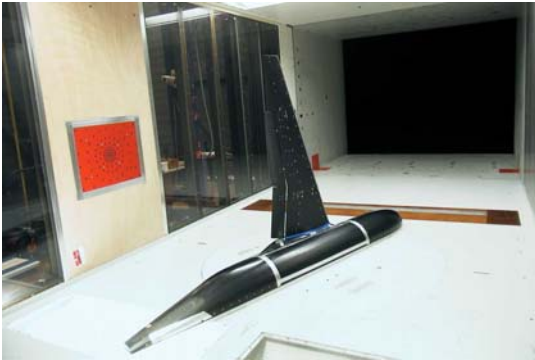
FIG 9. Typical microphone-array measurement setup in the low speed facility of DNW (DNW-LST). The DNW microphone array is mounted to the side wall of the test section.
