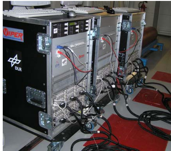
FIG 12. DLR data acquisition system. The picture shows three units which comprise 144 channels.
