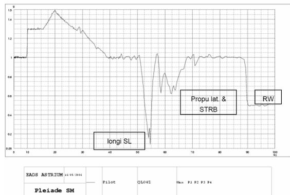
FIG 12. Structural Model – Z Sine Qualification
