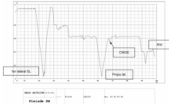
FIG 11. Structural Model – Y Sine Qualification
