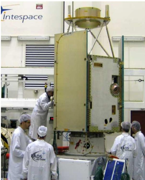
FIG 8. PLEIADES Structural Model – Longitudinal test
