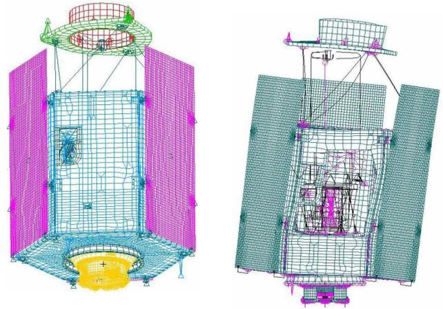
FIG 7. PLEIADES HR MEF – First lateral Mode @ 18Hz
