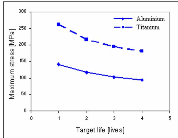
FIG 2. Loading Level for specified target life
