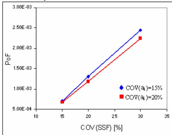
FIG 10. Probability of failure for combinations of scatter in  $a_i$  and  $SSF$  for case a)
