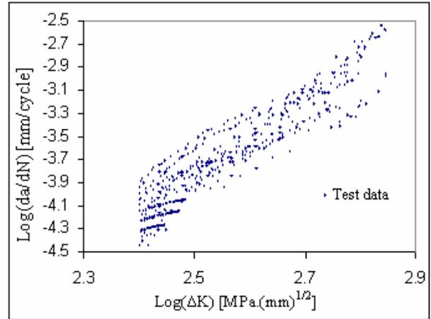
FIG 4. Crack growth rate data for similar Aluminium alloys (16 batches)
