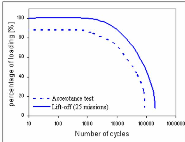
FIG 1. Exceedance curve for small ECLSS Equipments
