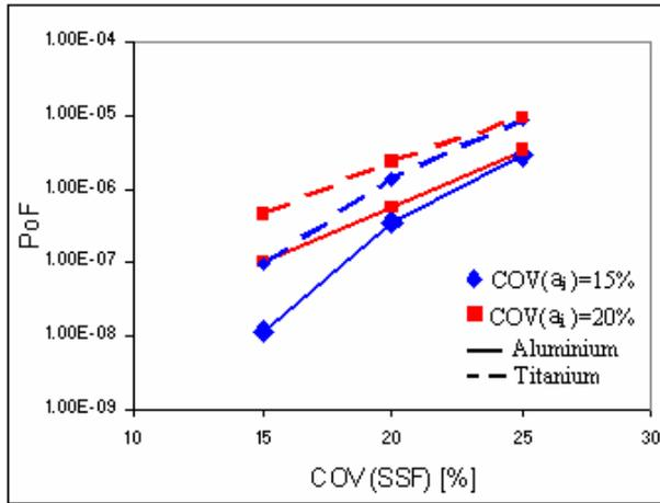
FIG 6. Probability of failure for combined scatter in  $a_i$  and  $SSF$
