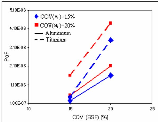
FIG 7. Probability of failure .vs. COV ( $SSF$ )
