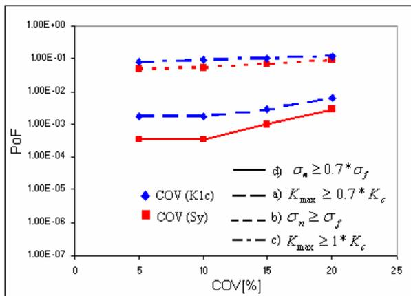
FIG 11. Probability of failure .vs.  $K_{Ic}$  or  $\sigma_{flow}$
