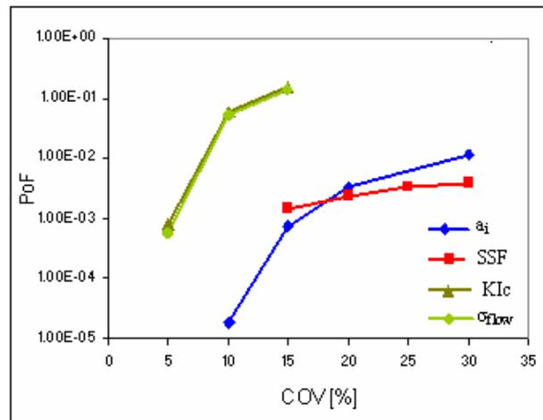
FIG 9. Sensitivity of PoF to crack depth, Stress Scaling Factor, fracture toughness and flow stress
