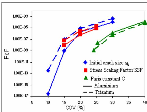
FIG 5. Sensitivity of PoF to crack depth, Stress Scaling Factor, Paris constant (Aluminium and Titanium alloys)
