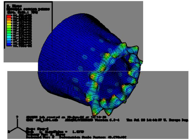
FIG 5. Buckling mode obtained with ABAQUS using a nonlinear prebuckling state ( $t = t_1$ ).
