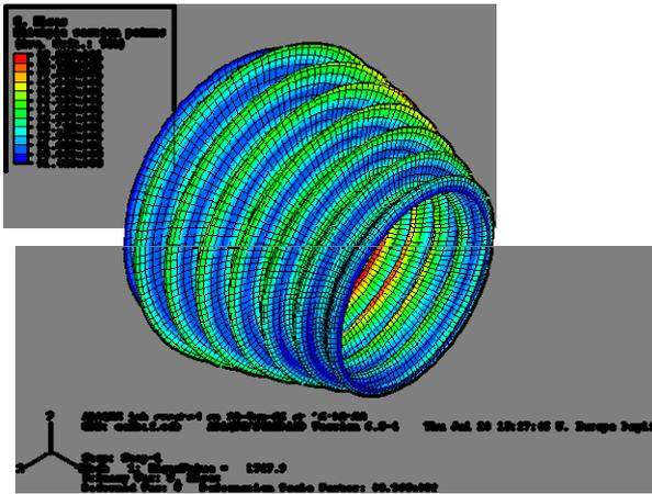
FIG 4. Buckling mode obtained with ABAQUS using a linear prebuckling state ( $t = t_1$ ).
