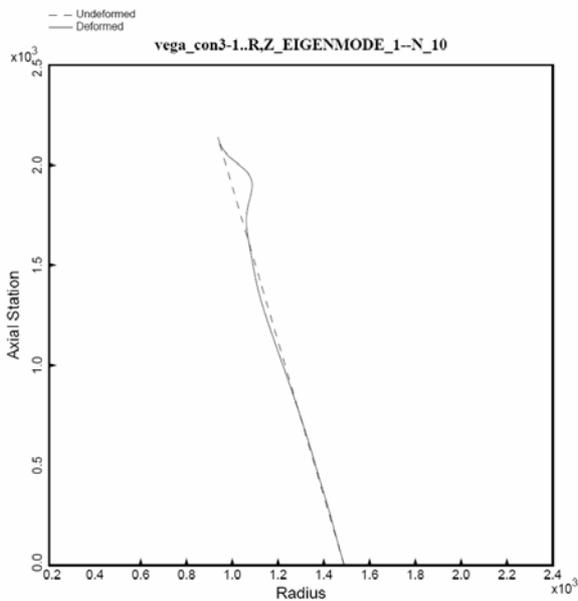
FIG 3. Buckling mode obtained with semi-analytical program BOSOR4 using nonlinear prebuckling ( $t = t_1$ ).
