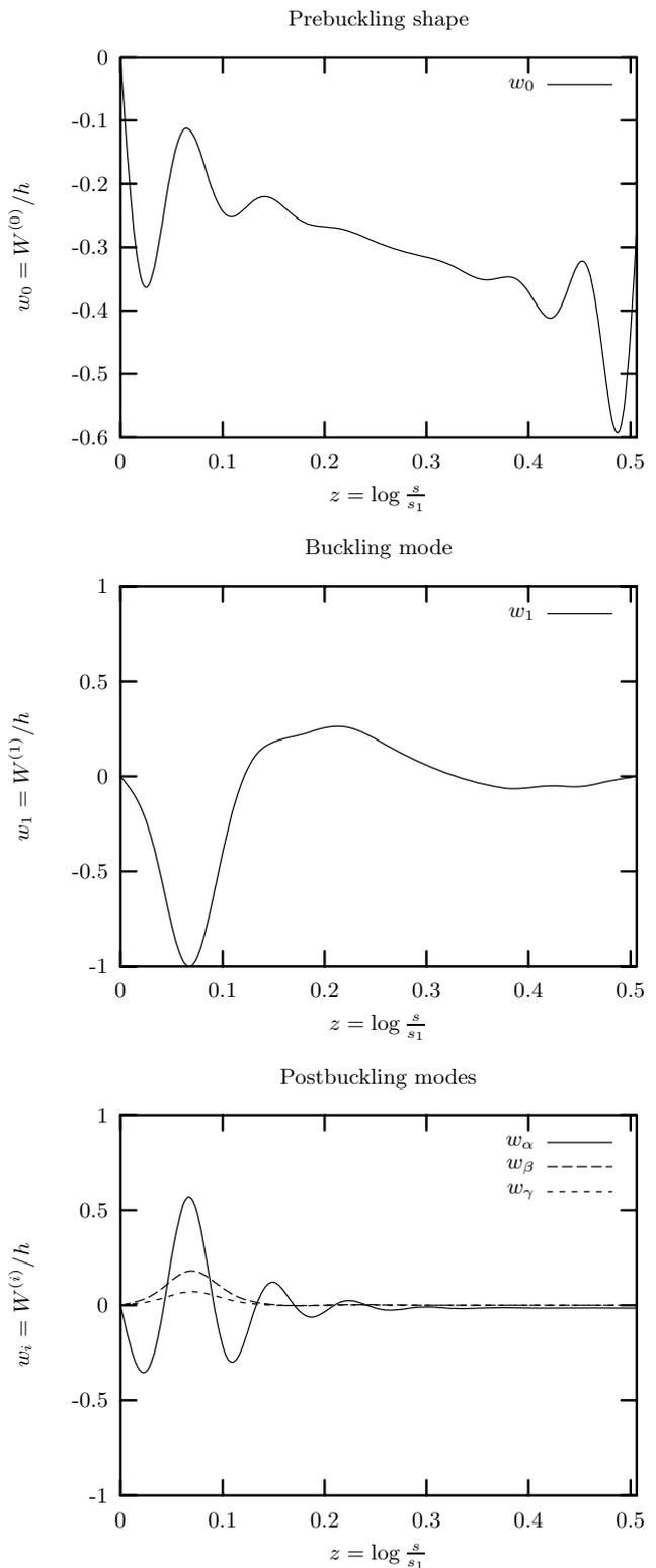
FIG 2. Prebuckling mode, buckling mode, and the different components of the postbuckling mode obtained with semi-analytical program BAAC using nonlinear prebuckling ( $t = t_2$ );  $s_1$  is the meridional coordinate at the top edge.
