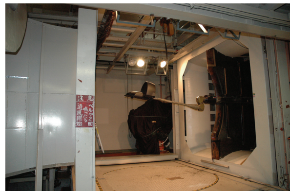
FIG 9. Wind tunnel test section
