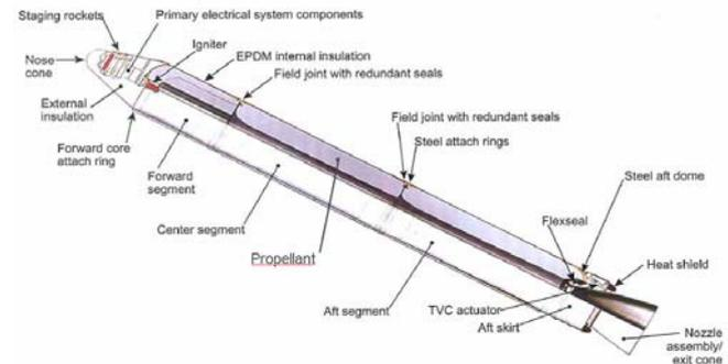
**Fig. 10: Typical cross section of a large SRM**
