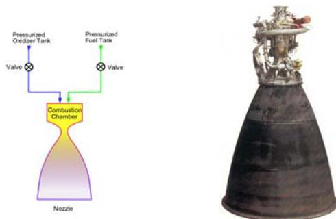
**Fig. 2: Left: Basic principle of a pressure-fed cycle. Right: Ariane 5 upper stage engine Aestus built by EADS Astrium at Ottobrunn.**
