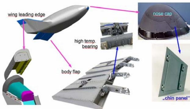
Fig. 20: Hot structural elements of a re-entry vehicle (courtesy MT Aerospace)
