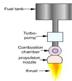
Fig. 1: Basic principle of liquid propulsion.
