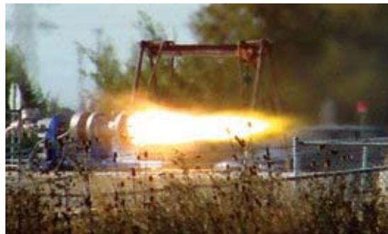
Fig. 14: LOX/Paraffin hybrid test at NASA Ames (Img.:NASA)
