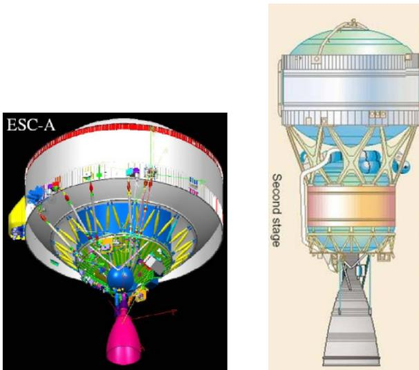
**Fig. 17: Ariane 5-ESC-A nested design and Delta IV Ø 5,1 m version, detached design**
