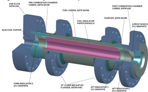
Fig. 12: SS1 hybrid motor schematic (Image NASA)
