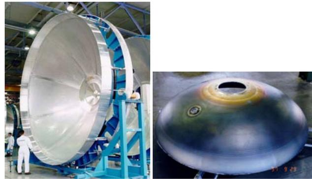
**Fig. 18: Large Tank Bulkheads: Gore-panel technique of Ariane 5 EPC Spinformed Dome for Japanese H II-A**
