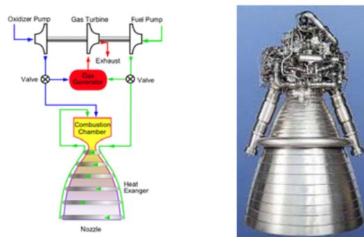
**Fig. 3: Left: Basic principle of a gas generator cycle. Right: Ariane 5 Vulcain 2 core stage engine.**
