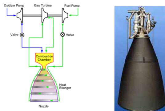
**Fig. 4: Left: Basic principle of an expander cycle. Right: Ariane 5 upper stage engine Vinci**
