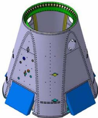
Fig. 21: XPERT hot metal TPS configuration with ODS metal cone, CMC nose and Flaps (Image Courtesy Dutch Space - EADS Astrium)
