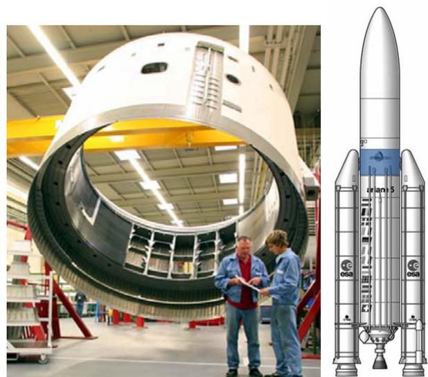
**Fig. 19: Ariane 5 front skirt of the main stage**
