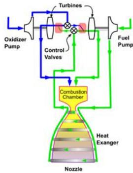
Fig. 6: Basic principle of a FFSCC.
