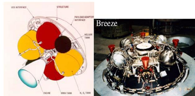
**Fig. 16: Ariane 5-EPS and Rockot-Breeze upper stage (courtesy IRS of Uni-Stuttgart)**
