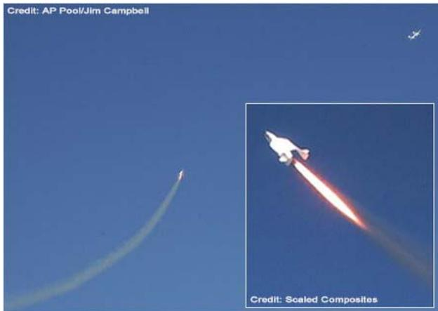
Fig. 13: SS1 hybrid motor in operation (Image courtesy J.Campbell & SC)
