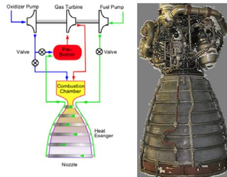
**Fig. 5: left: Basic principle of a staged combustion cycle.**
