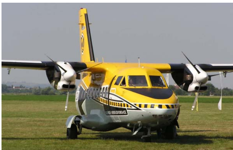
Fig.1 - L-410 Turbolet, twin engine 19-seats turboprop (produced by Aircraft Industries – former LET Kunovice)
