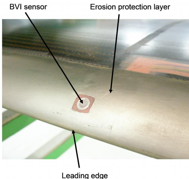
**FIG 2. BVI sensor is located at the leading edge of the rotor blade inside the erosion protection layer.**
