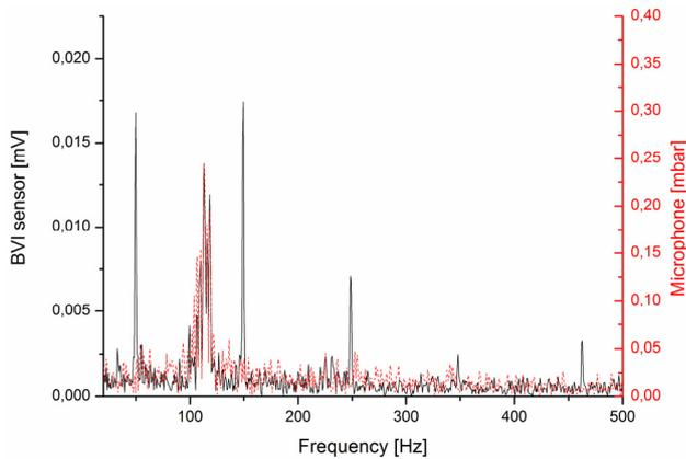
**FIG 7. Turbulence measurement amplitude spectrum at 20 m/s at 16.2° blade pitch angle.**
