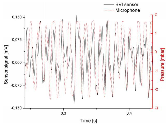
**FIG 5. Turbulence pressure signal versus time for an air velocity of 15 m/s at 6,1° pitch angle of the rotor blade.**
