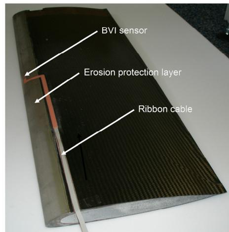
**FIG 3. EC145 rotor blade segment with integrated cable wiring.**
