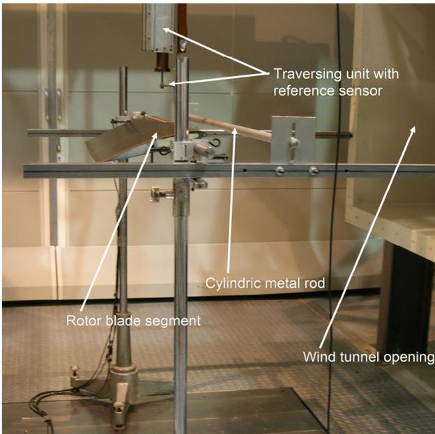
**FIG 4. Wind tunnel turbulence measurement set up.**
