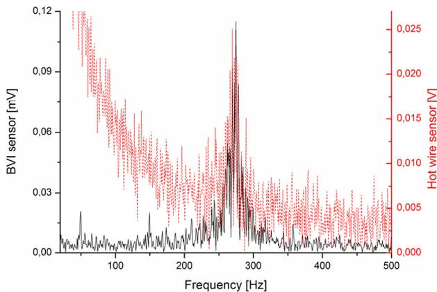
**FIG 8. Turbulence measurement amplitude spectrum at 50 m/s at 6.1° blade pitch angle.**
