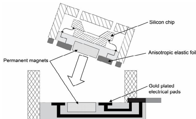
**FIG 1. Robust and easy-maintenance two-component MEMS package for rotor blade BVI sensor. Top: Replacable sensor capsule. Bottom: Permanently installed carrier.**
