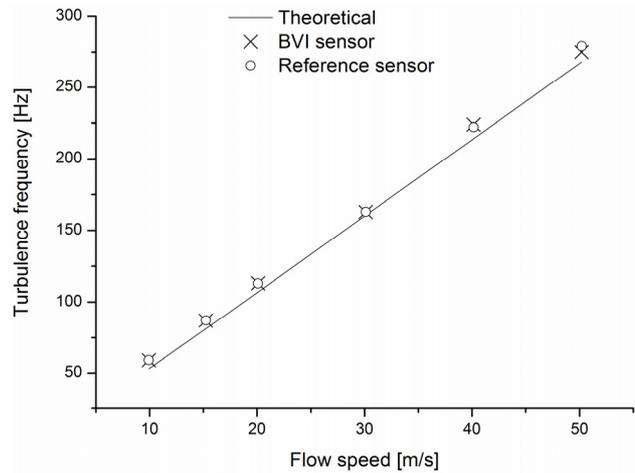
**FIG 9. Comparison between measured and theoretical turbulence frequencies at different flow speeds.**
