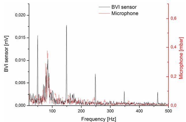
**FIG 6. Turbulence measurement amplitude spectrum at 15 m/s at 6,1° pitch angle of the rotor blade.**
