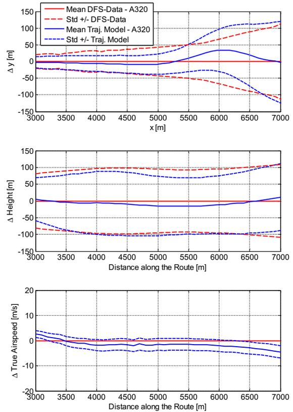
FIG 12: A320 trajectory model quantities referred to DFS data
