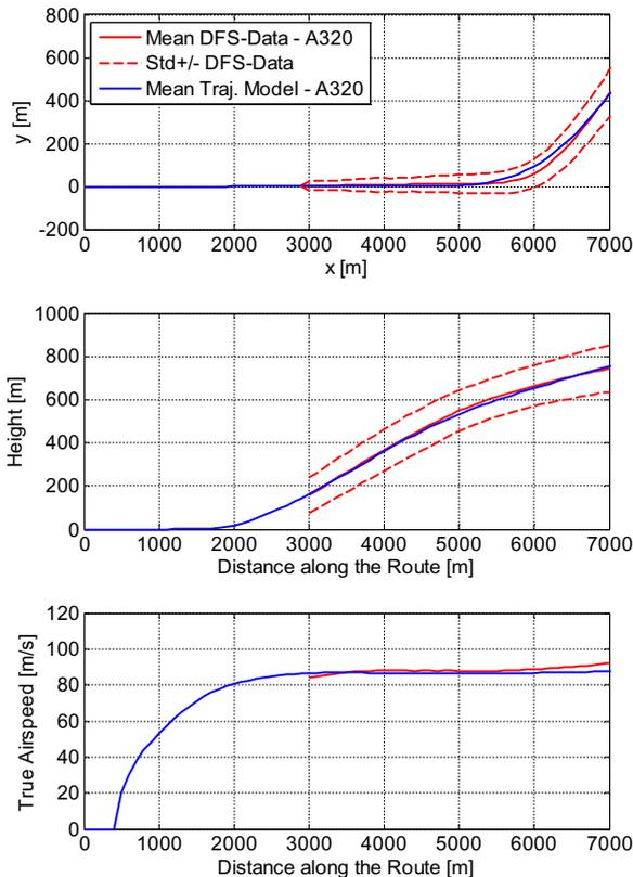
FIG 10: A320 lateral, vertical and speed profile
