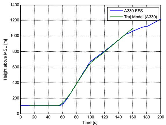
FIG 8: Height above MSL from A330 FFS versus trajectory model (A330)
