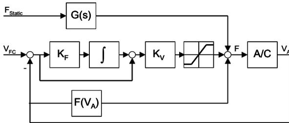
FIG 3: Thrust control
