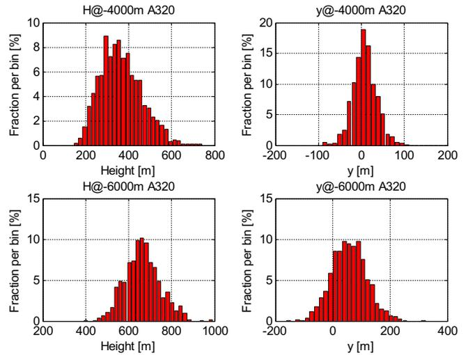
FIG 11: Distribution of height and lateral offset for 1000 A320 departures at 4000 m and 6000 m (DFS data)
