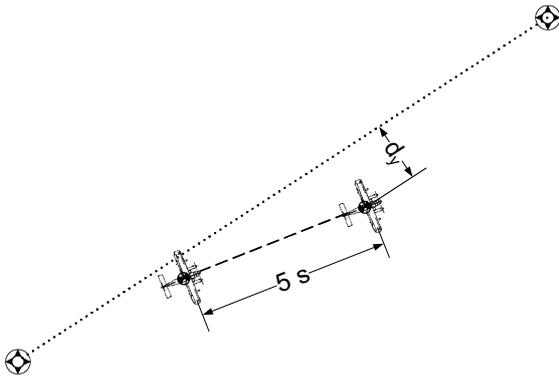
FIG 2: Flight path deviation to a straight segment
