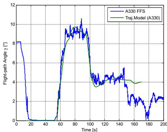
FIG 6: Flight path angle from A330-FFS versus trajectory model (A330)
