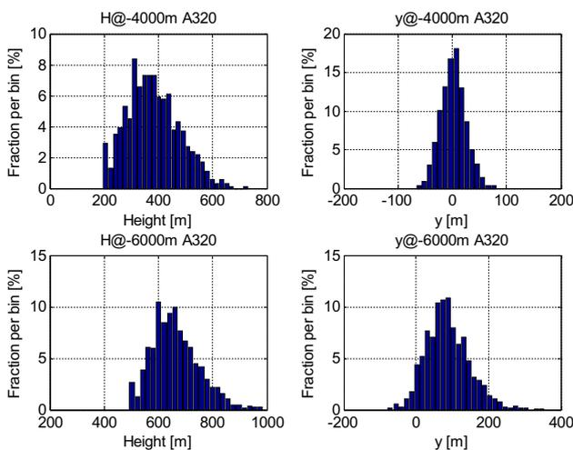
FIG 13: Distribution of height and lateral offset for 1000 A320 departures at 4000 m and 6000 m (TM data)
