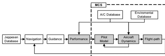
FIG 1: Modules of the Trajectory Model
