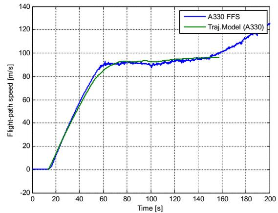
FIG 7: Flight path speed from A330 FFS versus trajectory model (A330)
