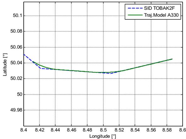
FIG 9: Lateral trajectory A330-300
