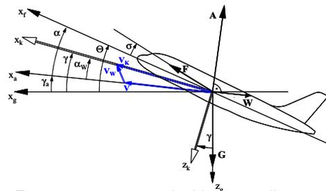
FIG 14: Forces, moments, velocities, coordinate system, and angles in the x-y-plane [4]
