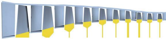
FIG 9. Flow channel feature-based generated HPC of NASA E<sup>3</sup> engine
