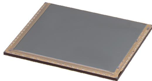
FIG. 12 Infrared Focal Plane Array (here: 640 x 512 pixels)
