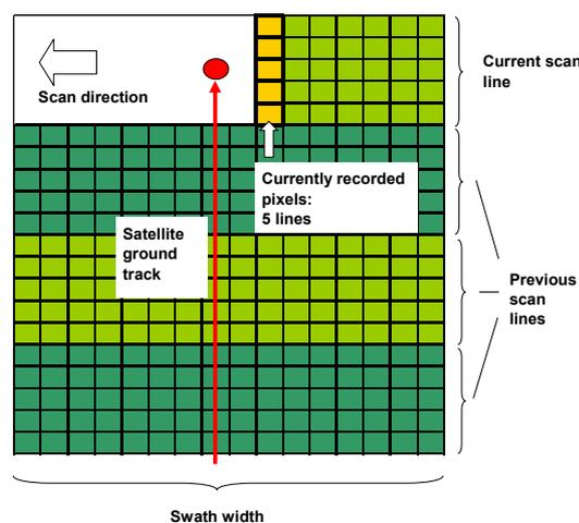
**FIG. 1: Recording pattern of a rotating scanner with multiple pixel lines per scan**
