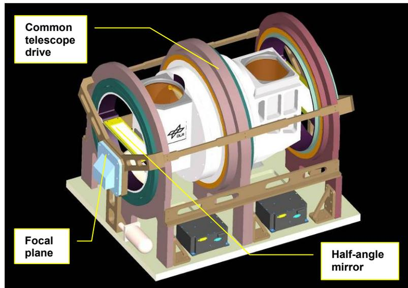
FIG. 16: Design of a METimage instrument with visible and infrared light processed separately, therefore with two apertures. A common structure and common telescope drive provide good synchronisation and a compact design.
