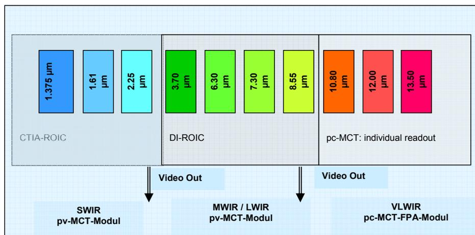
**FIG. 8 METImage Infrared Focal Plane assembled as MCM consisting of 3 basic infrared submodules.**
