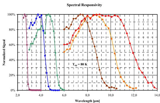
FIG. 9 Adjustment of MCT-infrared sensors in accordance to system requirements
