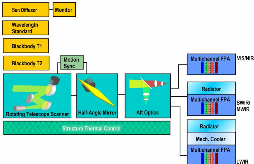
FIG. 15: *Advanced configuration of a METimage instrument*
