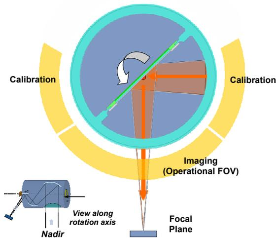
FIG. 3: Different portions of the field-of-view (FOV) are used for imaging and calibration, without the need for additional mechanisms to move calibration sources into the optical path or interruption of normal operation.
