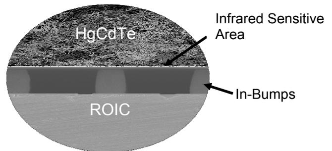
FIG. 13 Cross section of MCT-Focal Plane Array: Indium bumps providing electrical, thermal, and mechanical interface between MCT and ROIC (diameter of In-bump  $\square$  10 µm), the infrared light is impinging MCT from the back side.
