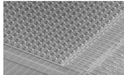
FIG. 11 ROIC, provided with Indium bumps for flip chip mounting
