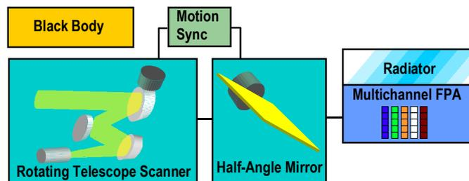
FIG. 14: *Basic configuration of a METimage instrument*
