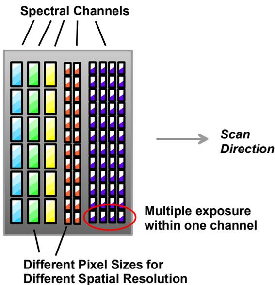
**FIG. 6: Detector arrangements in the focal plane**
