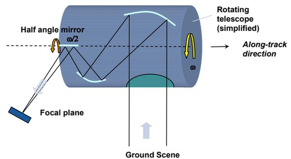
**FIG. 2: Simplified principle of a rotating telescope scanner**
