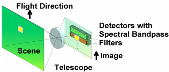
**FIG. 5: In-field separation of spectral channels**
