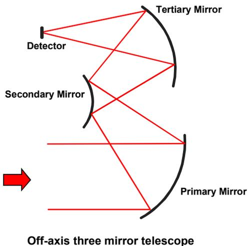
FIG. 4: Two different basic designs of mirror telescopes. The off-axis triple mirror design needs more elements, but this introduces additional degrees of freedom for image enhancement. The "central obscuration", leaving the central portion of the primary mirror in the two-mirror design without function and deteriorating the image quality, can be avoided.
