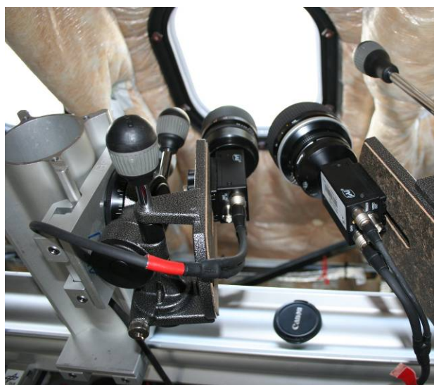
FIG 1. EDT cameras mounted on XS95 profile beam behind the A/C window.
